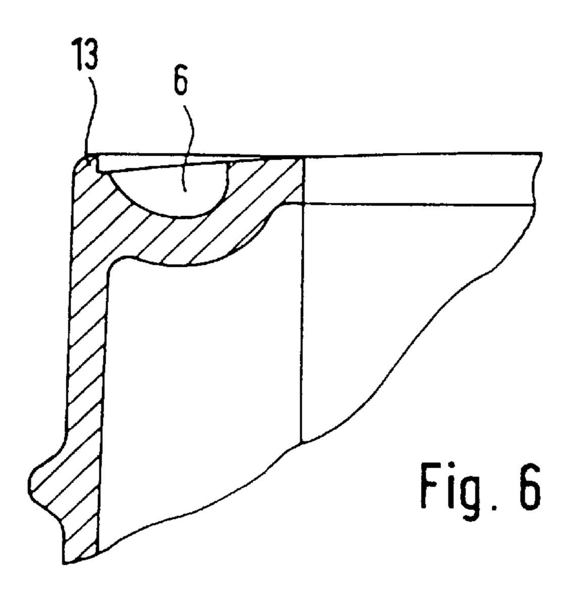
The present invention pertains to a pot-shaped heat exchanger with a front-side connection to a burner or the like for accommodating a burner flame tube, a lateral water inlet 5 in the bottom of the pot and a water outlet in the area of the
