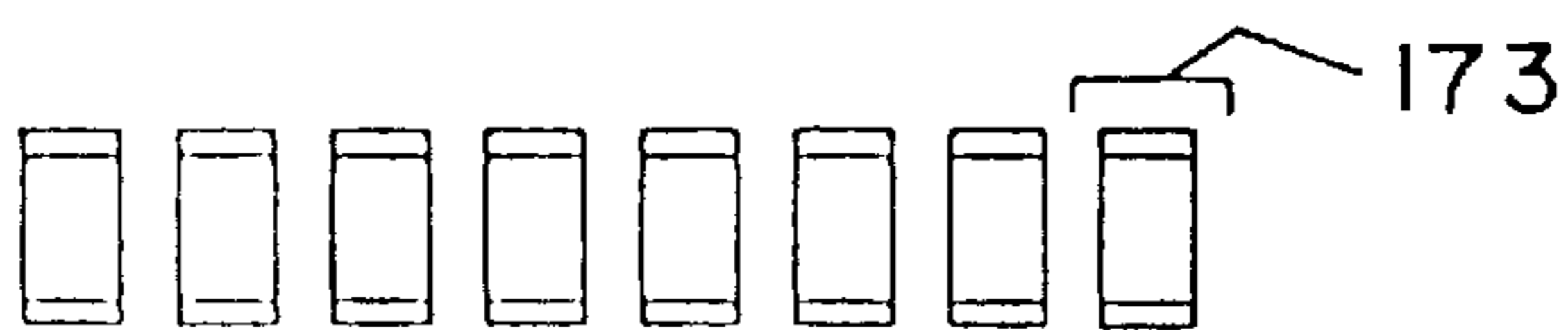
F I G . 1 7 C CROSS SECTION OF THE THERMOMATERIAL CHIPS WITH THE LAYERS FOR SOLDERING.
