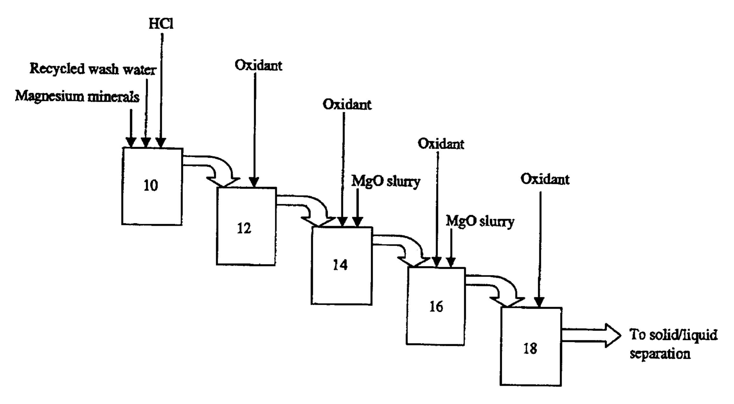
Figure 1: Leach and Neutralization Circuit
