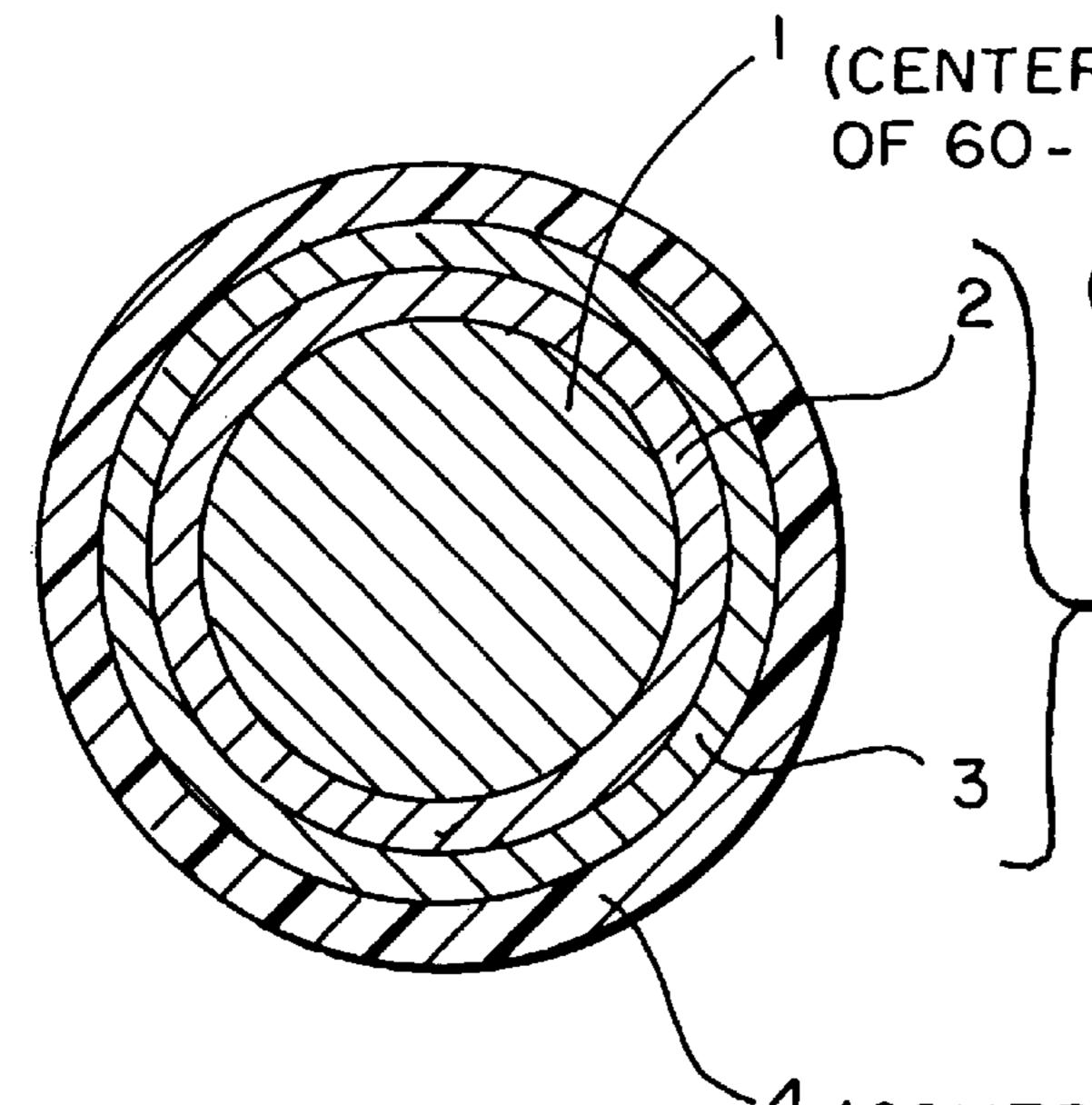
(CENTER HAVING JIS-C HARDNESS OF 60-80 AND DIAMETER OF 15-30mm)
