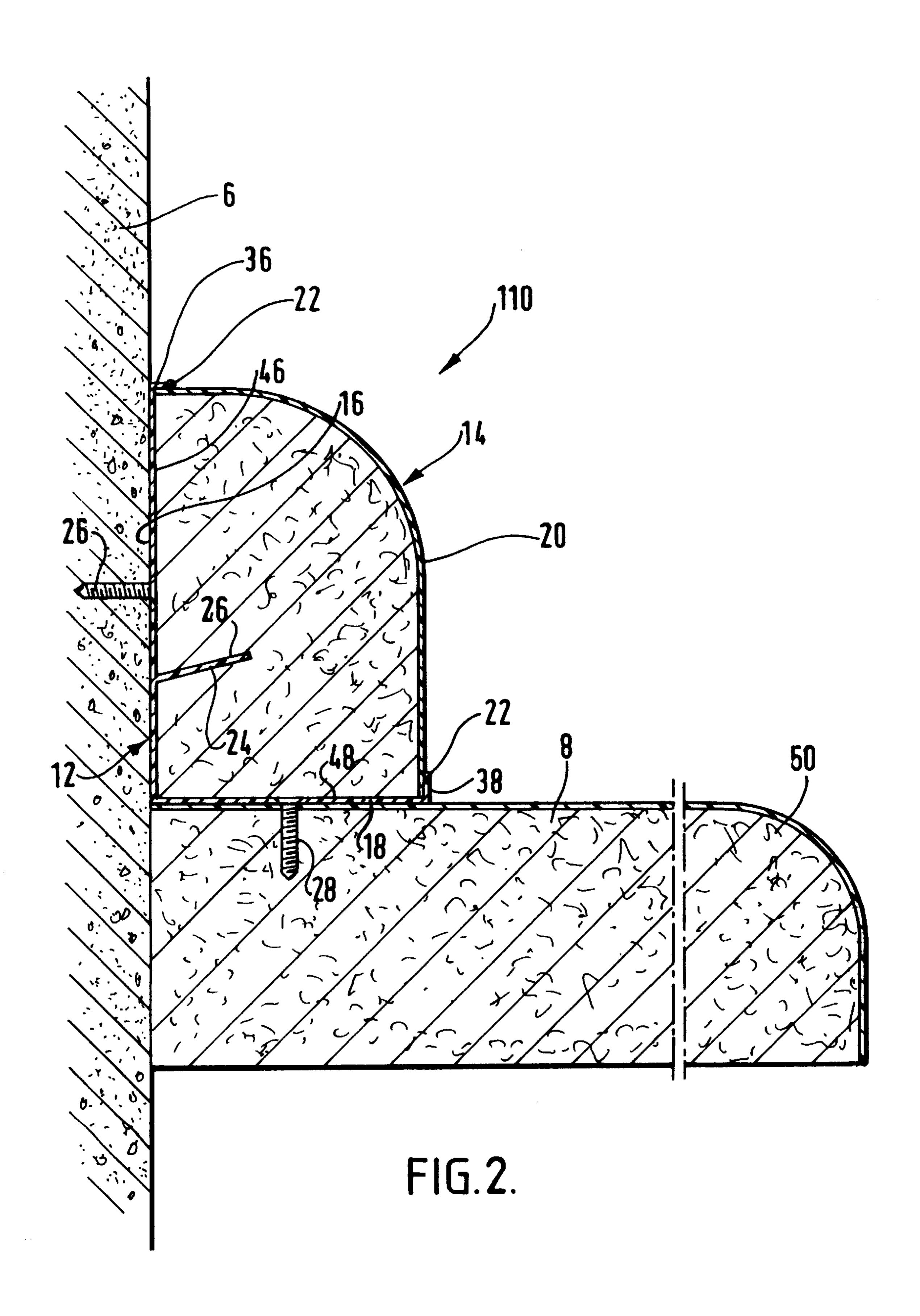
The present invention relates to an upstand assembly, particularly but not exclusively to an upstand assembly for a worksurface of a kitchen.
