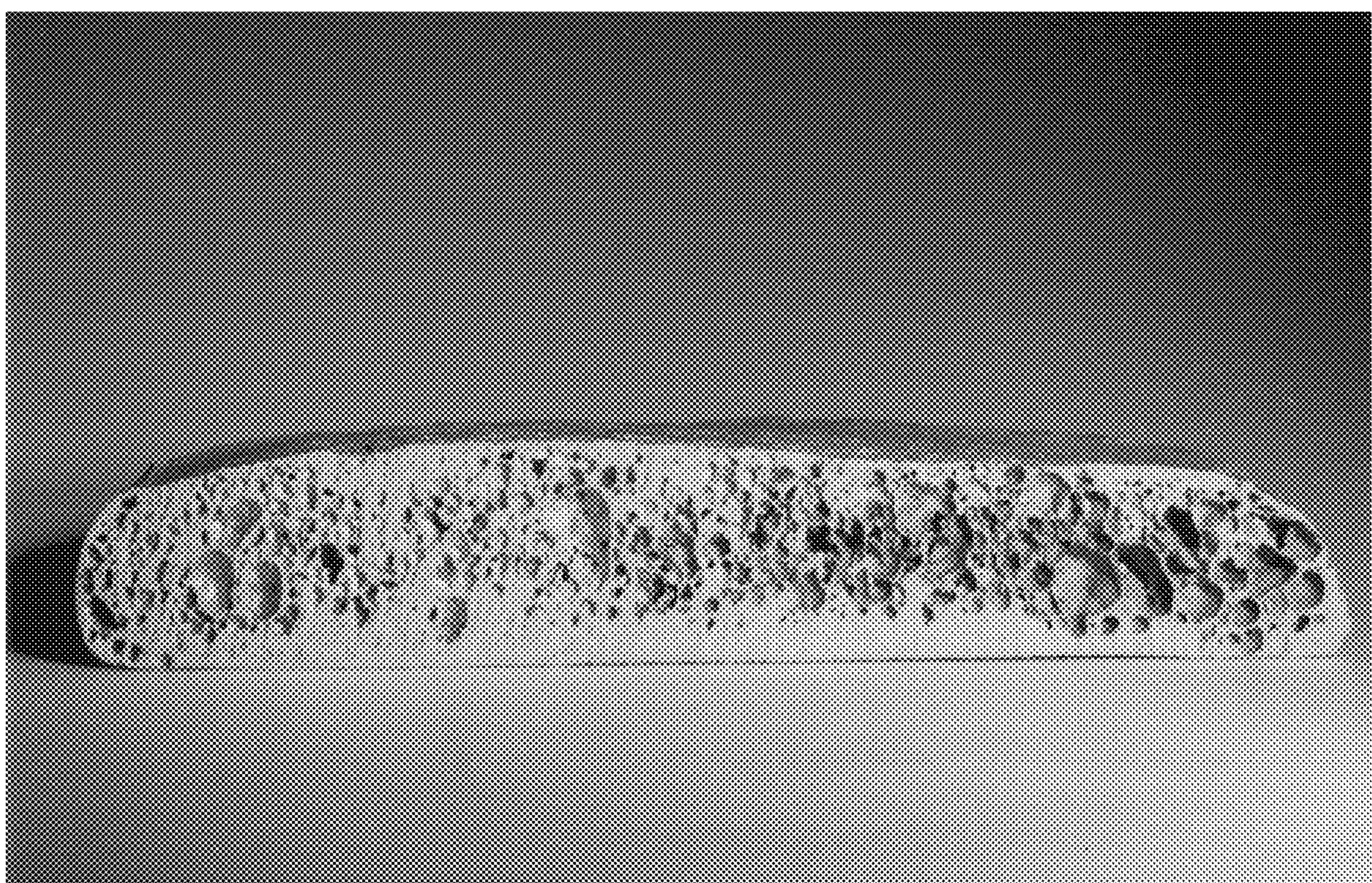
Aluminum foam produced with 0.5m % titanium hydride
