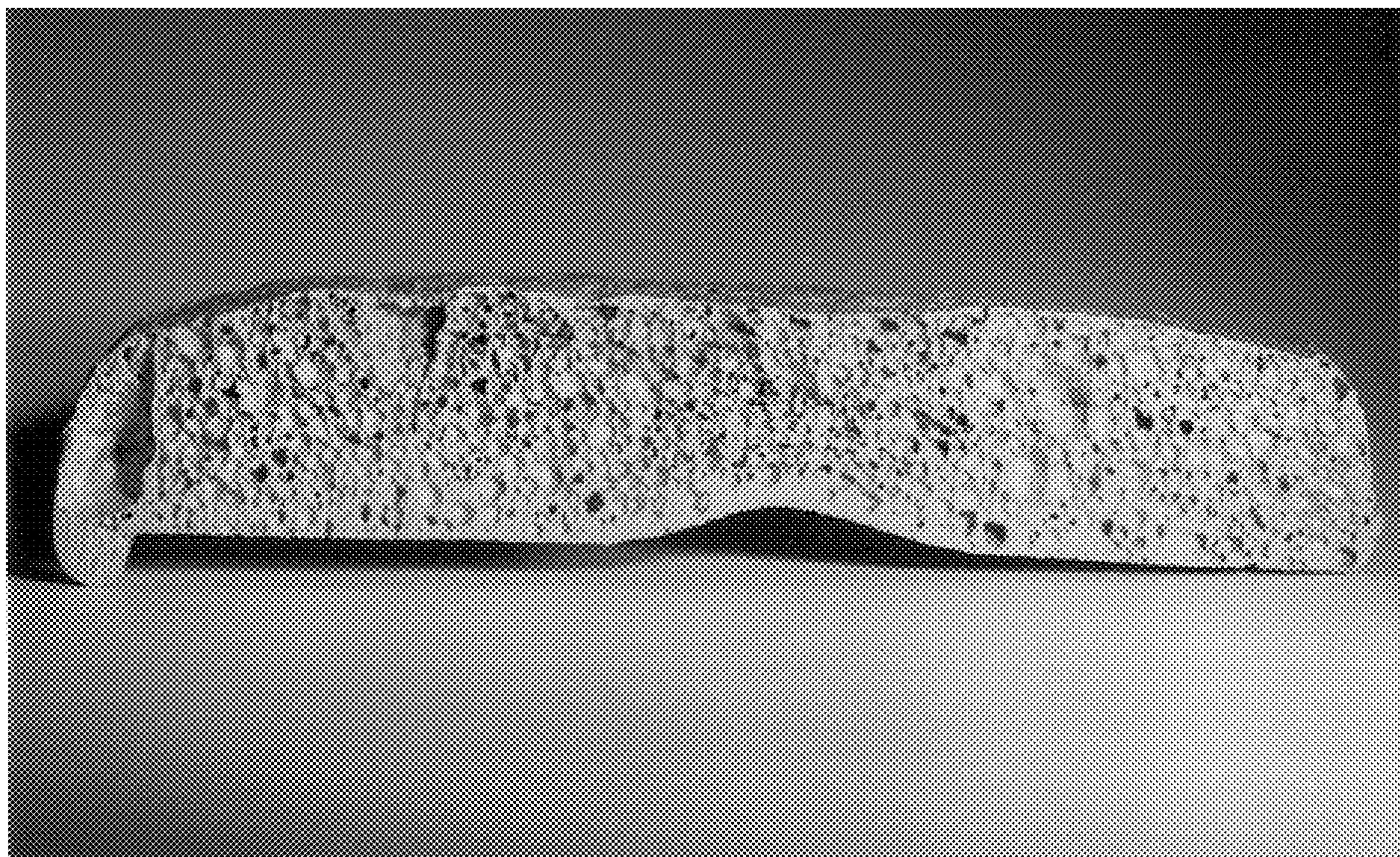
Aluminum foam produced with 0.5 m % magnesium hydride
