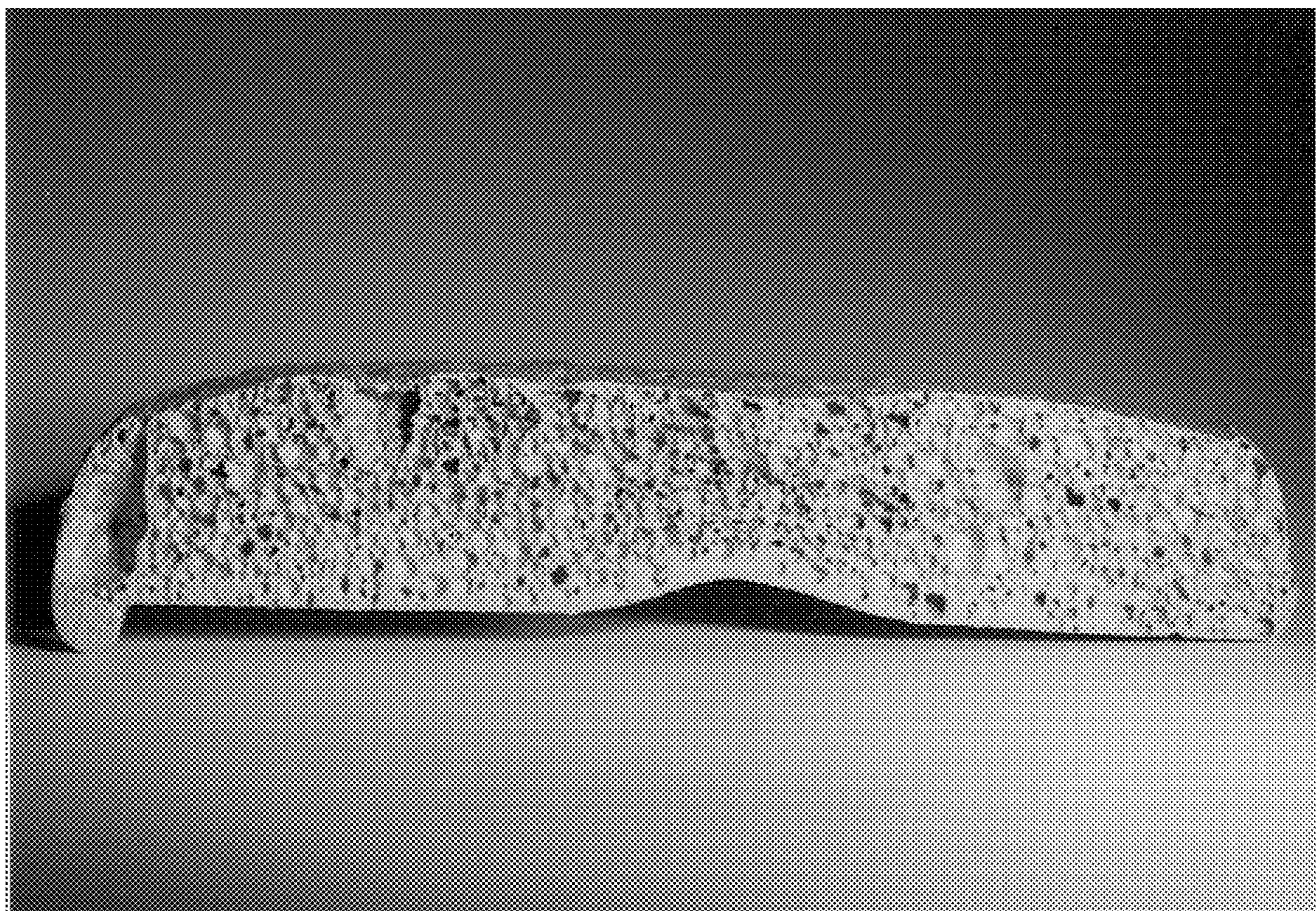
**Aluminum foam produced with 0.5 m % magnesium hydride
