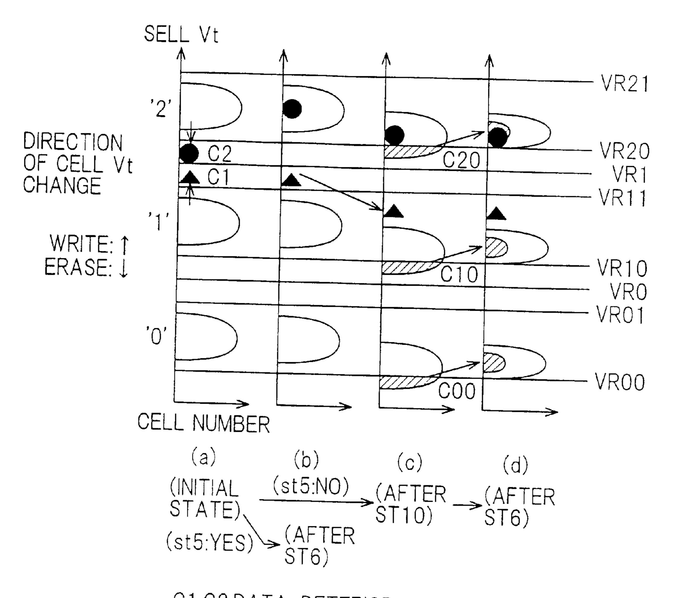
C1,C2:DATA-DETERIORATED CELL VR0,1:CELL Vt JUDGEMENT LEVEL IN READING DATA VRi0,i1(i=0-2):CELL Vt JUDGEMENT LEVEL IN DETECTING THE DETERRIORATION OF DATA AND WRITING DATA
