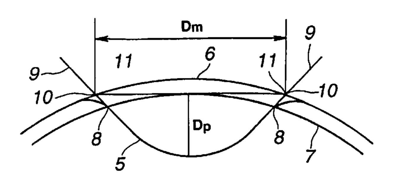
TWO TYPES OF DIMPLES 370 - 450 AT LEAST 63% OF BALL SURFACE DIMPLE VOLUME  $V_D > 4$  COVER S.P. 0.90 - 1.18 COVER GAGE 0.5 - 3.0mm
