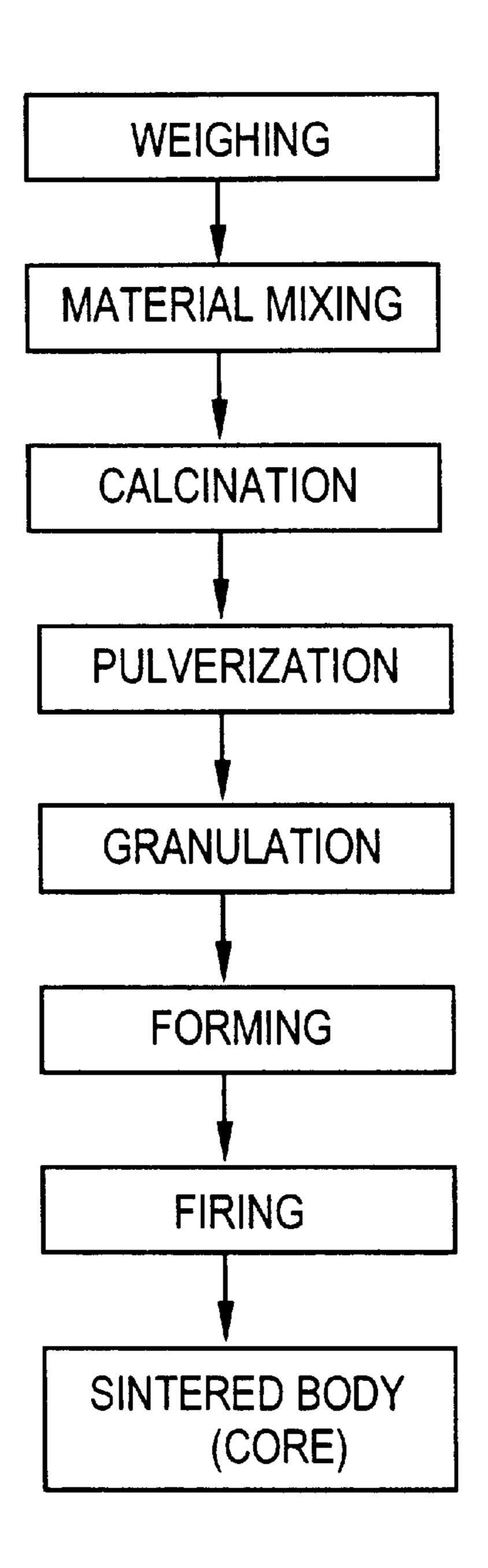
\* WHEN ALUMINA MATERIAL IS USED FOR CORE MATERIAL, SOME STEPS INCLUSIVE OF CALCINATION, AND PULVERIZATION STEPS MAY OFTEN BE DISPENSED WITH.
