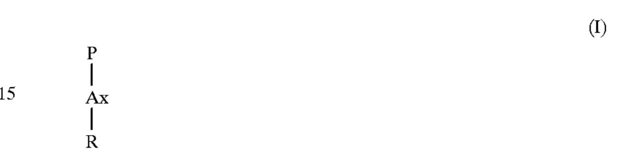
wherein P is a polymerisable unit, whereto the R—N—O group can be attached to, or wherein the R—N—O group forms part of the polymerisable unit or a combination of both.
