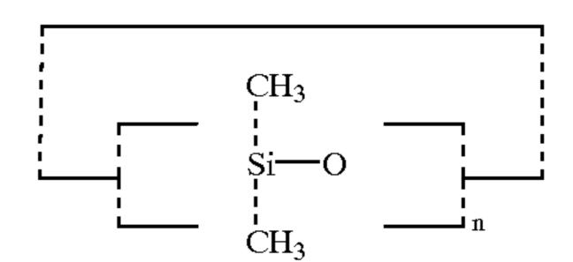
wherein n=1-7. Volatile linear polydimethylsiloxanes are also suitable and generally have from about 2 to 9 silicon atoms and are of the formula:
