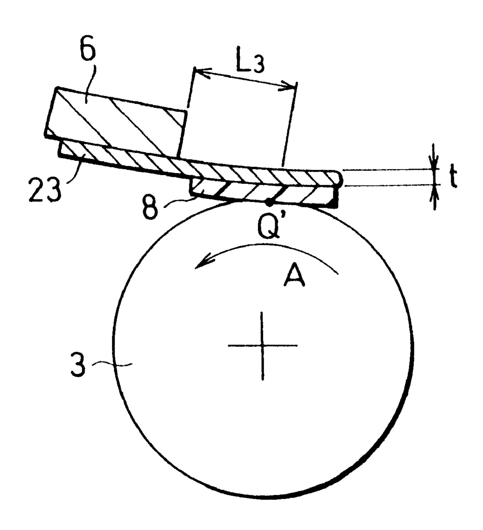
$L_3$ = 22 mm  $t_3 = 0.2 \, \text{mm}$
