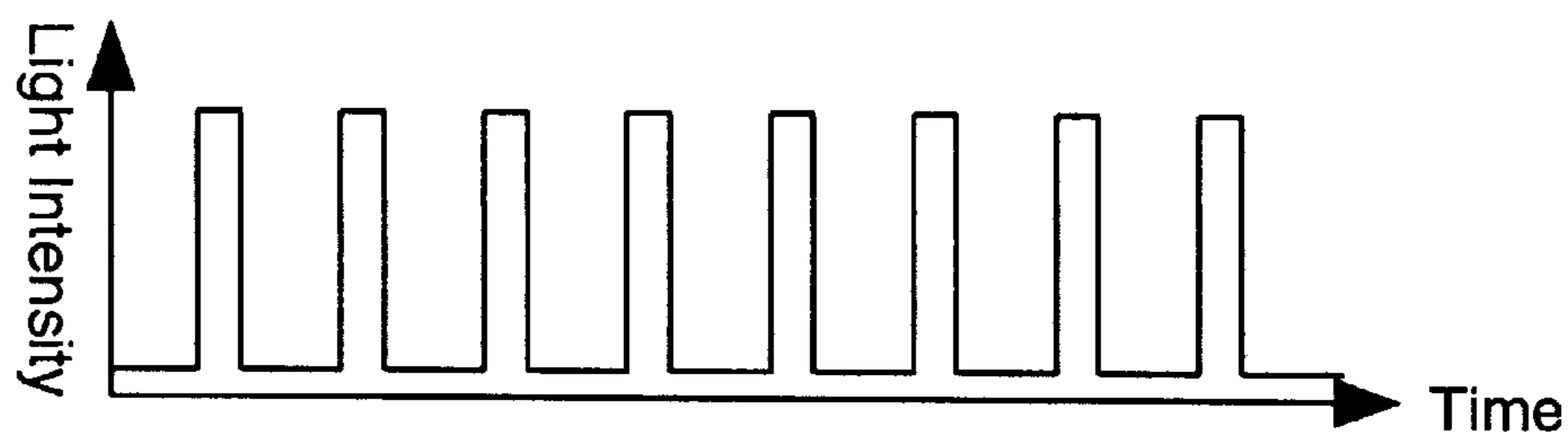
FIG. 7(2) Original signal light 16 (clock frequency f_0 < f_1 )
