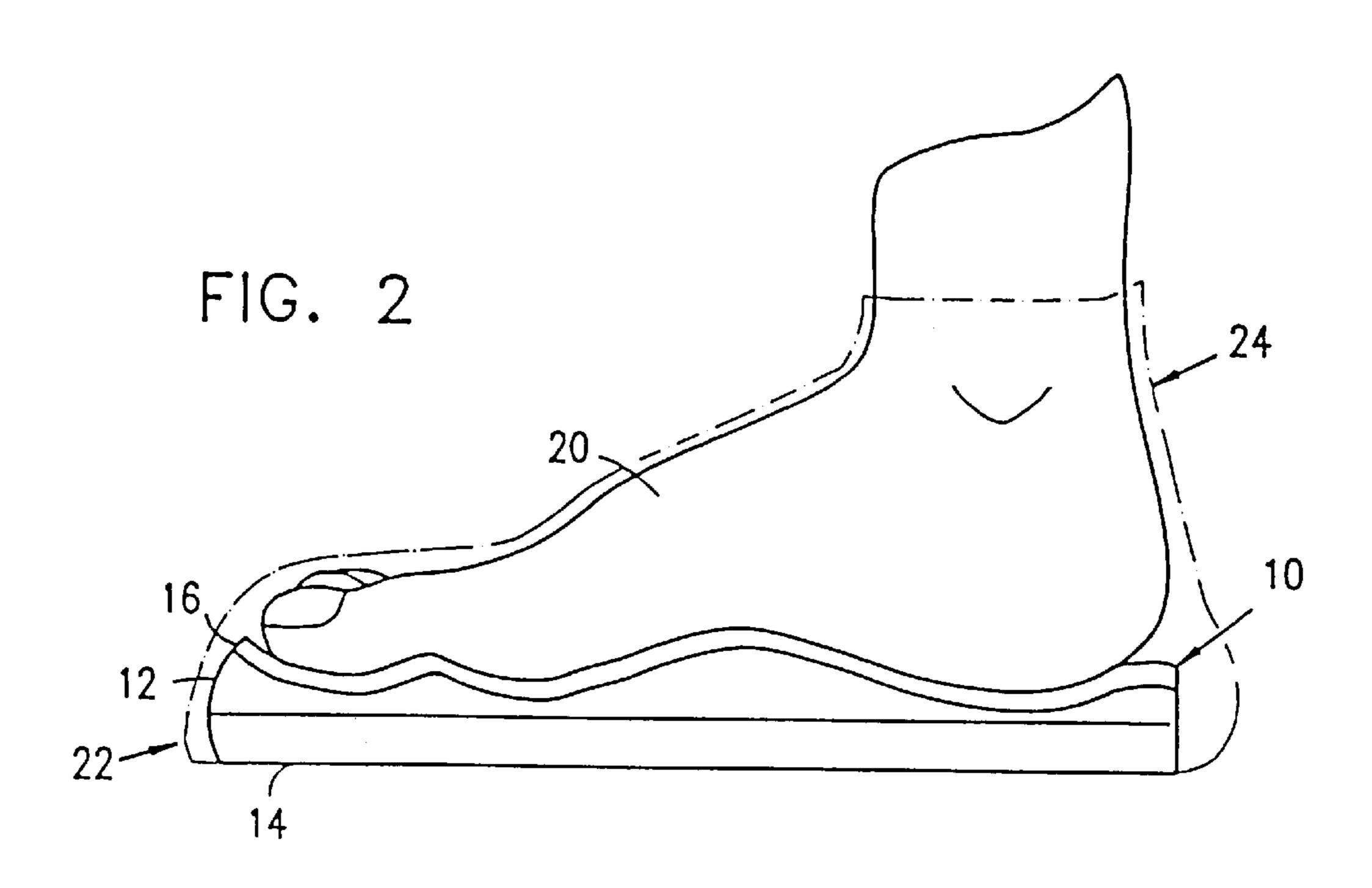
The present invention relates to insoles generally and more particularly to custom insoles which are directly molded by pressure from a user's foot.
