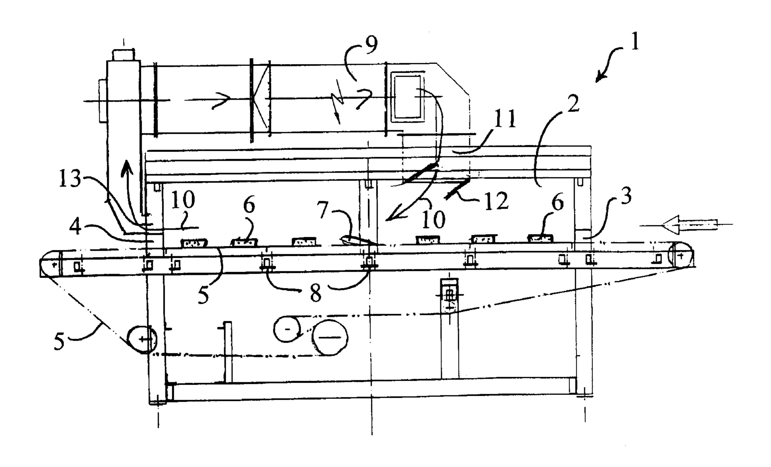
The invention relates to a cooking process and a cooking machine for exercising the process. More specifically, the invention refers to a method for continuously heat treating a 5
