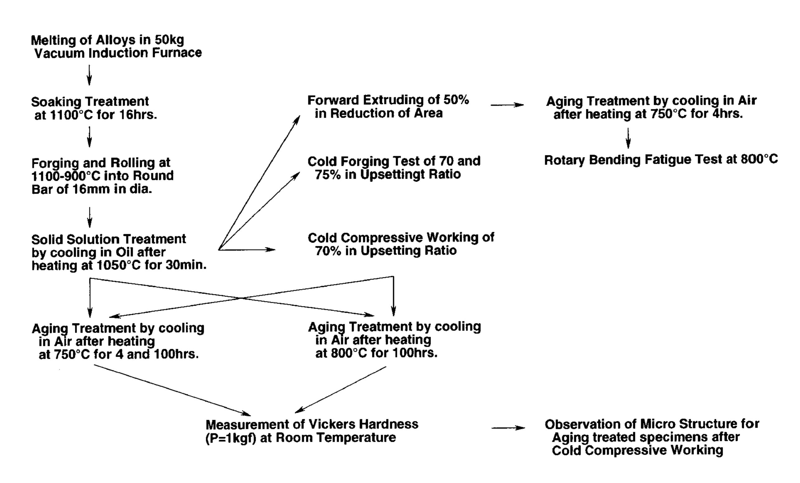
Melting of Alloys in 50kg Vacuum Induction Furnace
