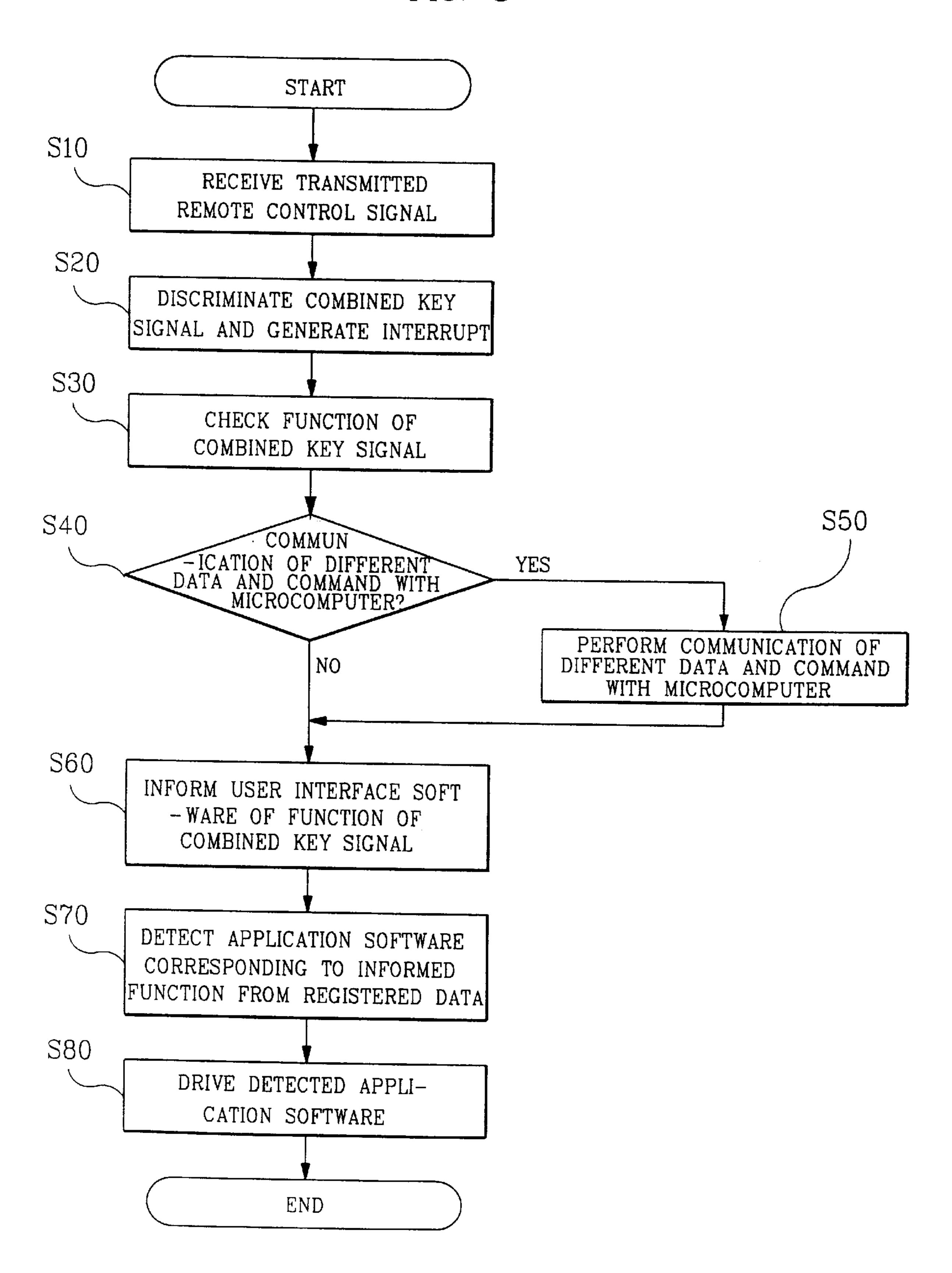
SYSTEM FOR REMOTELY CONTROLLING A COMPUTER HAVING A USER INTERFACE SOFTWARE COMMUNICATING WITH A DEVICE DRIVER AND DRIVING AN APPLICATION SOFTWARE TO PERFORM OPERATION BASED ON A COMBINED KEY SIGNAL
