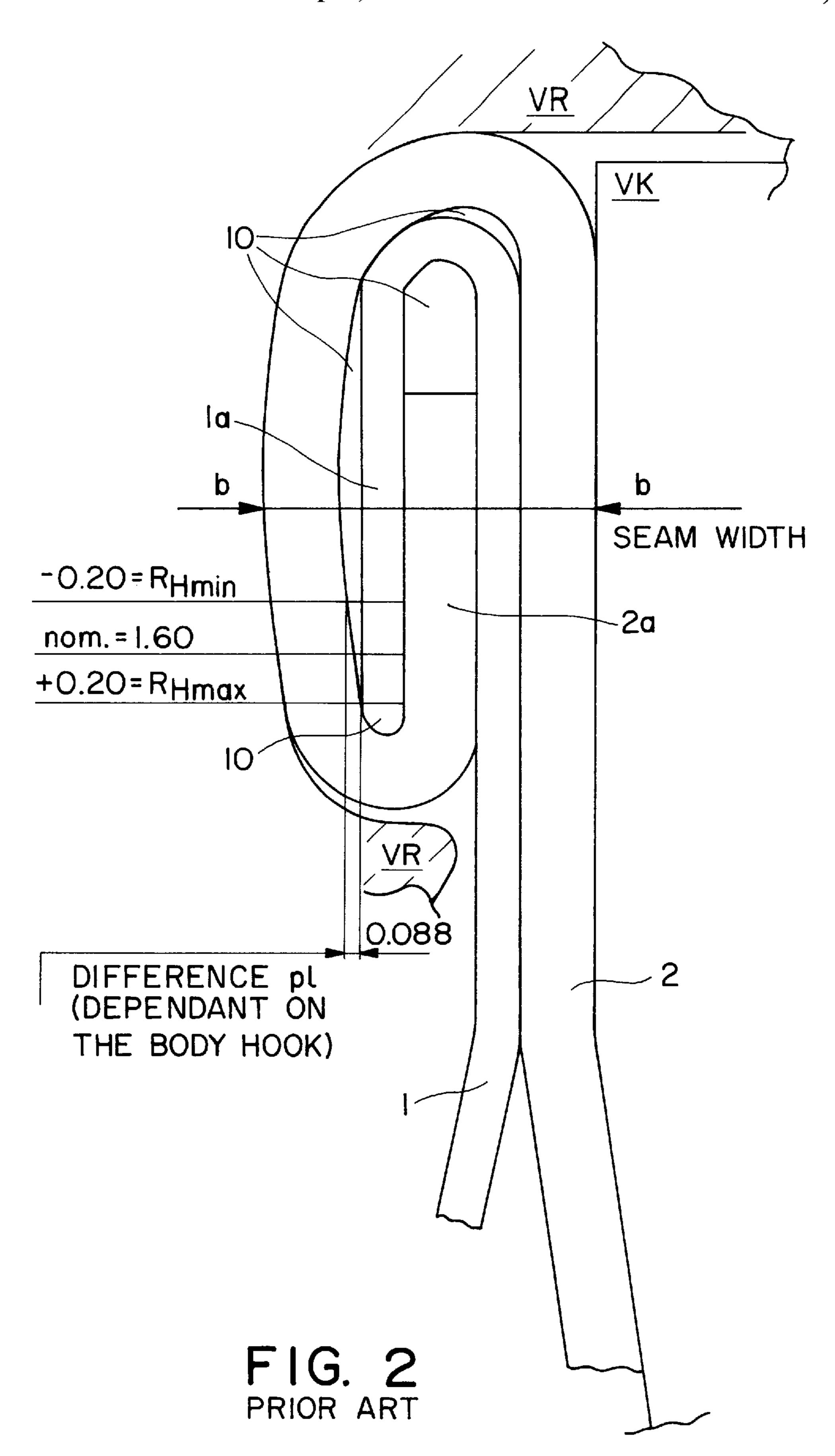
The technical field of the invention is the providing of a seam on a can body closed with a (can) end, such as beverage or food can made from sheet material. The function of such a seam is to hold the can end and the can body tightly together to protect them also against relatively high forces possibly becoming effective from outside, e.g. by pressure or shock, and from inside, e.g. by high or low pressure, and moreover, to hermetically air-seal the content of the can.
