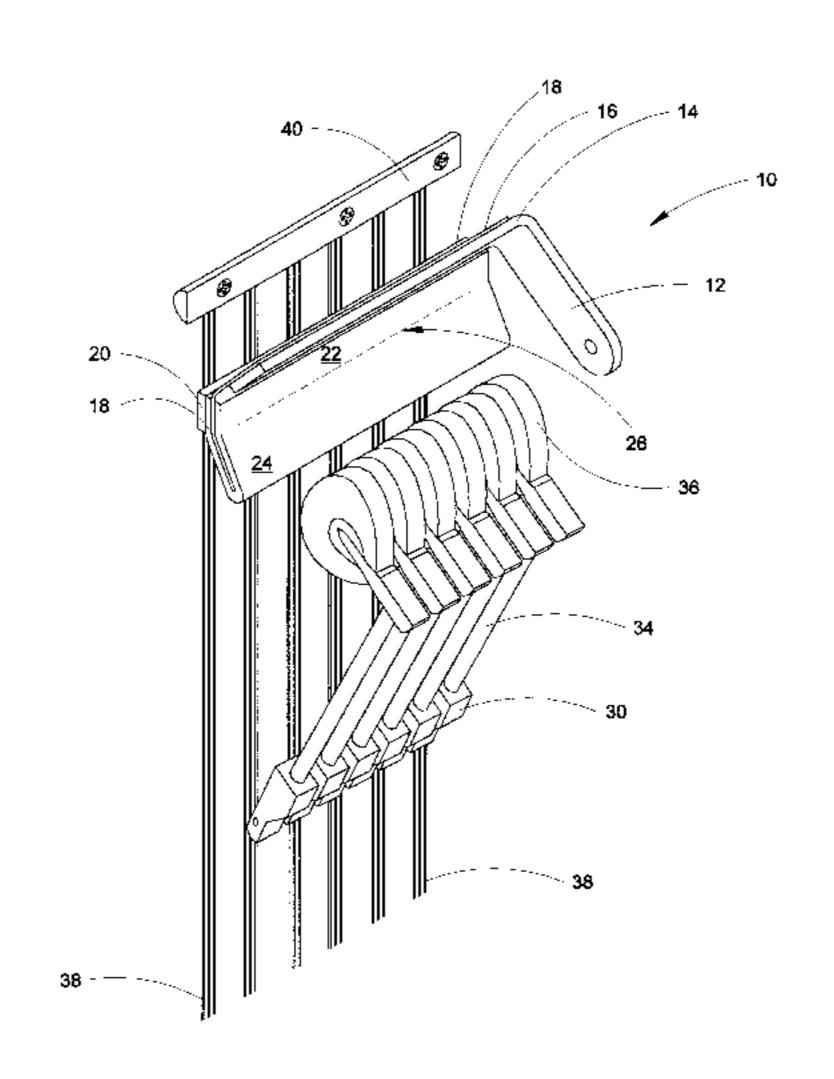
material, such that when the hammer head impacts the stop rail, the deflectable member somewhat displaces, as the hammer head impacts against this member. The hammer head stop rail also includes a sound and vibration absorbing pad that is brought into position against the strings of the piano, thereby tending to dampen any acoustic vibration that may otherwise become induced in the strings.
