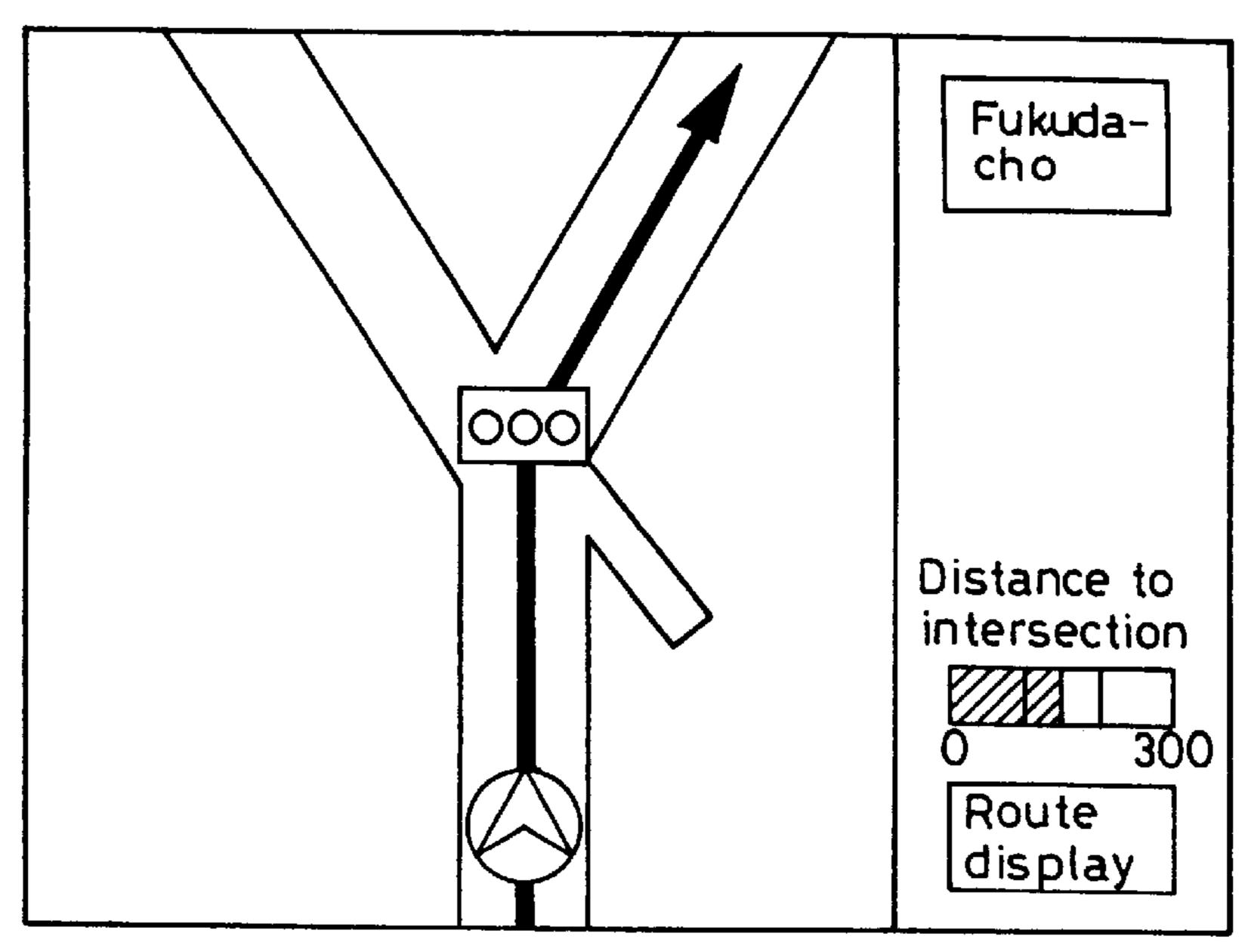
"Beep. Take the diagonally rightward direction at Fukuda-cho, which is about 300 meters ahead."
