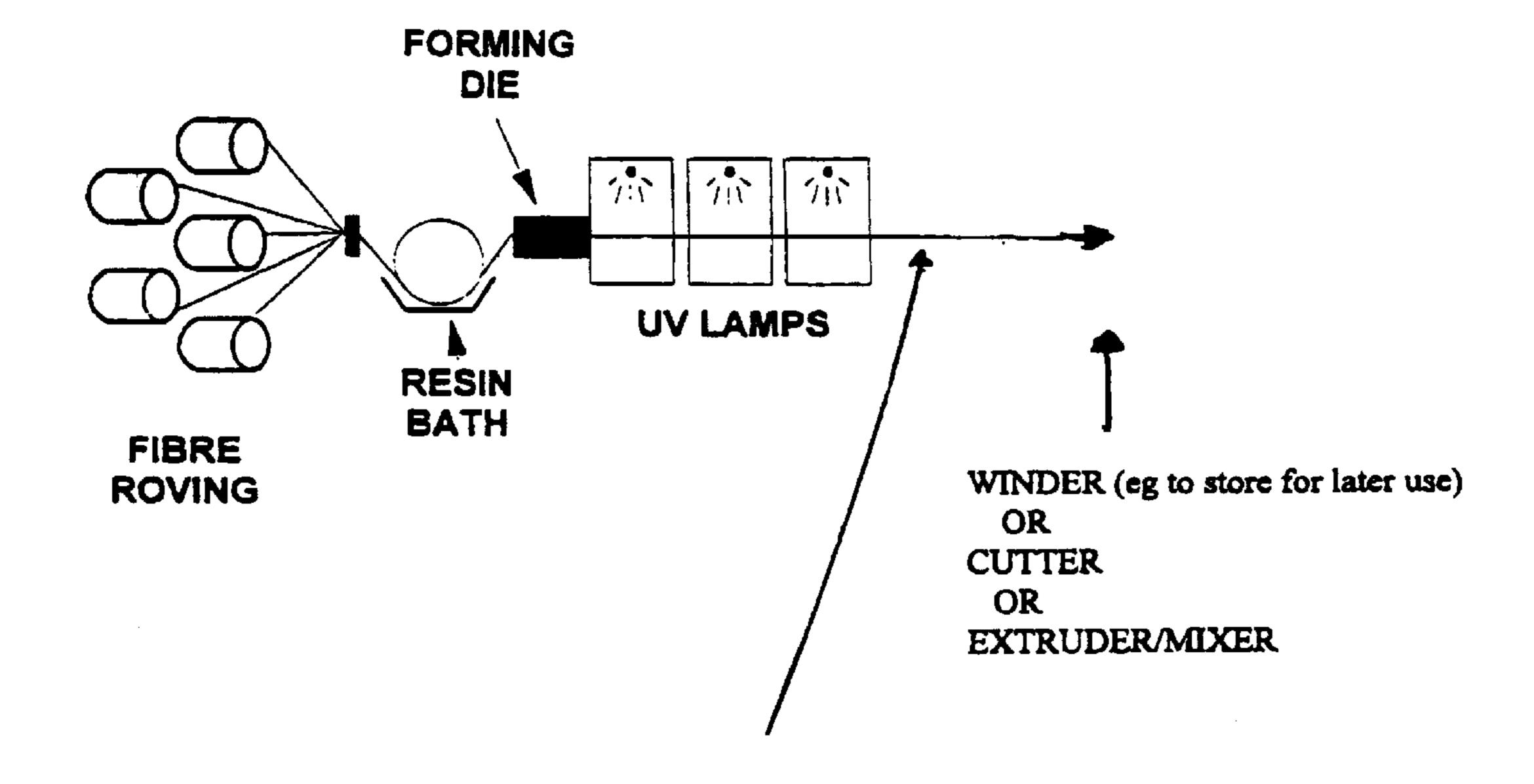
RADIATION POLYMERISED/IMPREGNATED FIBRE -RESIN INTERMEDIATE
