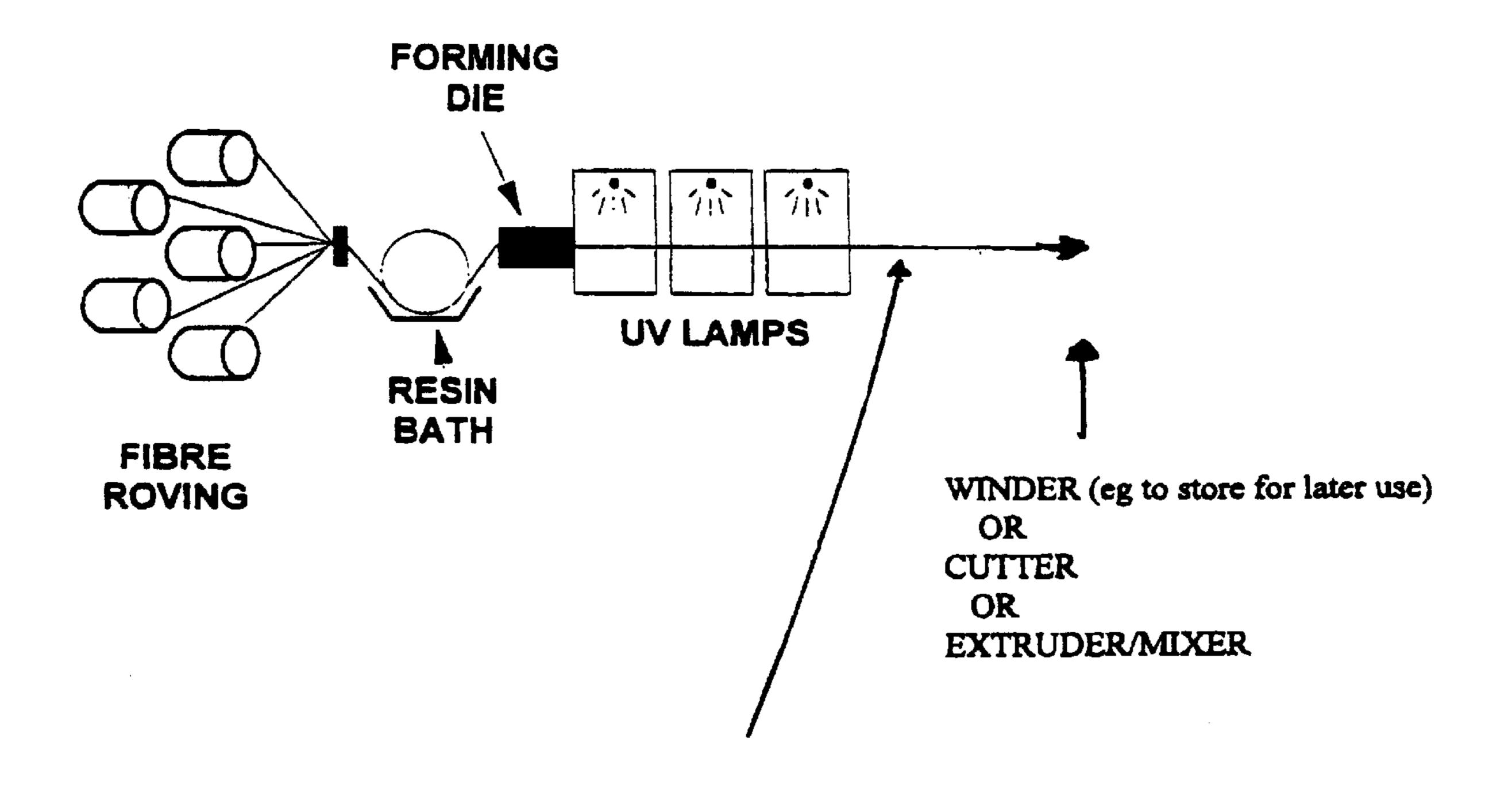
RADIATION POLYMERISED/IMPREGNATED FIBRE -RESIN INTERMEDIATE
