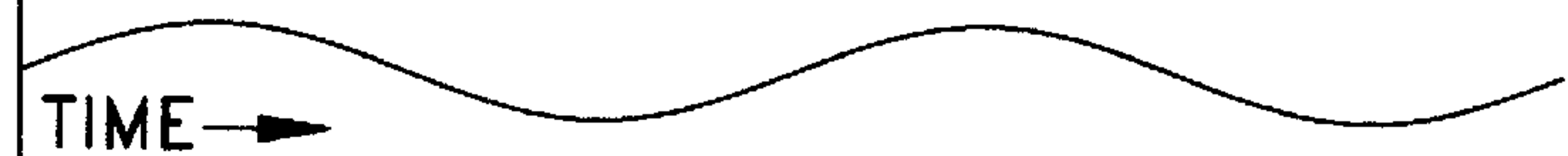
FIG. 14D DIESEL GENERATOR CURRENT 25% RATED
