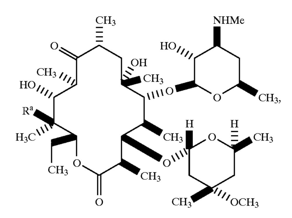
wherein R<sup>a</sup> is H or OH, by stepwise addition of iodine and base to the N-dimethyl-4"-deoxyerythromycin, preferably, accompanied by sparging with an inert gas.
