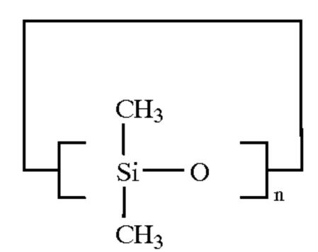
wherein n=1-7. Volatile linear polydimethylsiloxanes are also suitable and generally have from about 2 to 9 silicon atoms and are of the formula:
