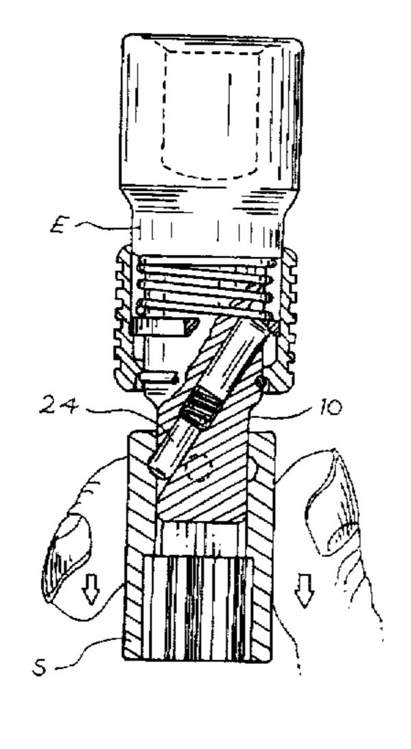
spring biases the sliding surface toward the pin, and a second, weaker spring biases the pin toward the sliding surface. Movement of the actuating member along the longitudinal axis of the drive stud in a selected direction
