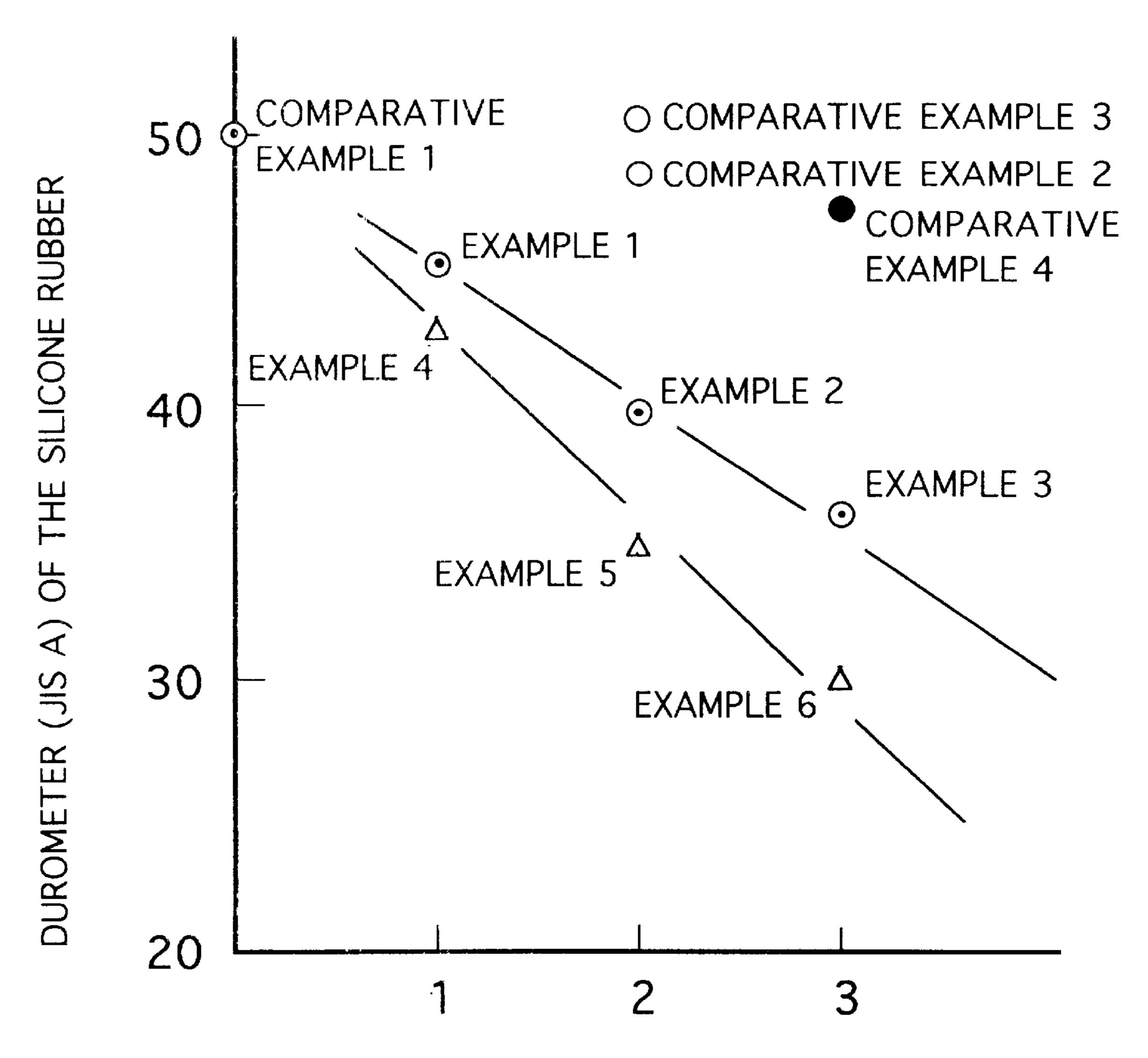
ADDITION (WEIGHT PARTS) OF ORGANOSILOXANE PER 100 WEIGHT PARTS SILICONE RUBBER BASE (I)
