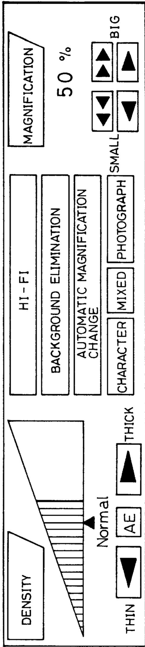
FIG. 7(b) POST-PROCESS SETTING SCREEN
