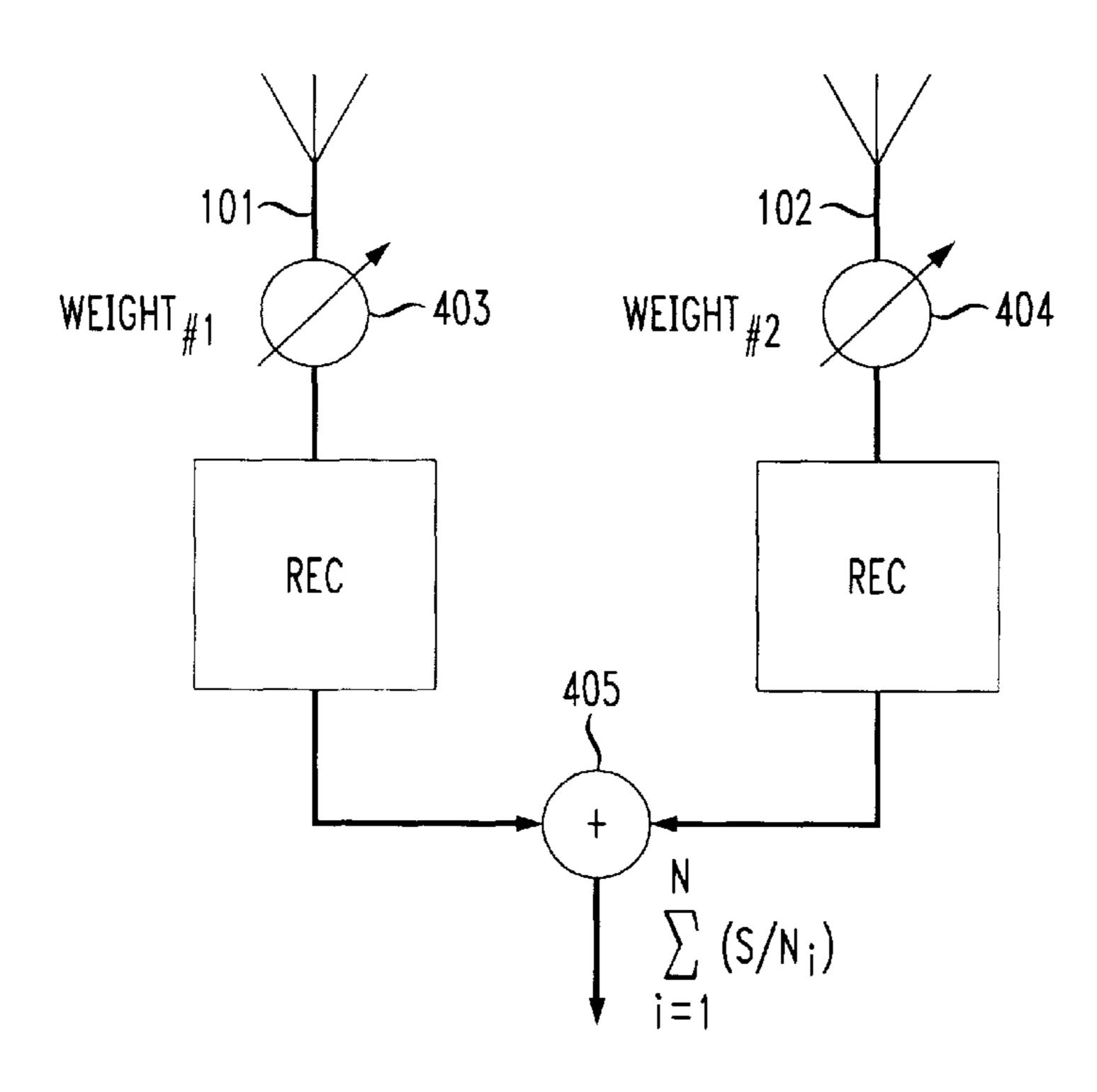
FIG. 4D EQUAL-GAIN COMBINING
