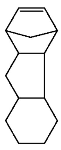
(wherein the lower 6-membered ring structure may have a double bond) and hydrogenating the polymer so that the hydrogenation rate of double bond in the main chain is at least 98% and the hydrogenation rate of the 6-membered ring structure is at least 90%.
