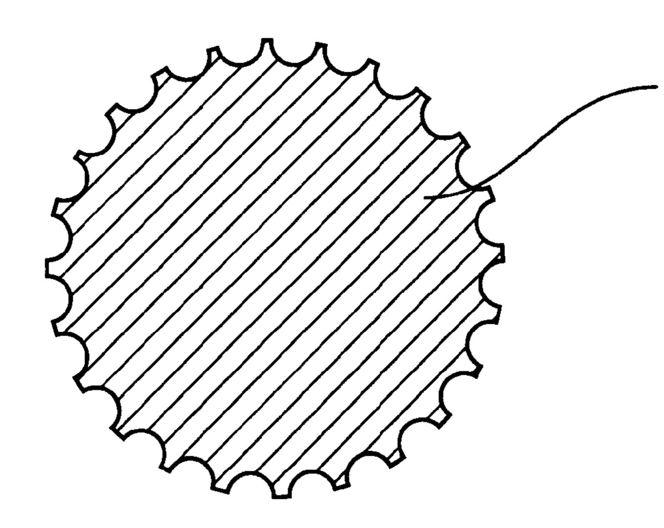
ONE-PIECE GOLF BALL CONTAINING FIBROUS ALUMINUM BORATE WHISKERS, PREFERABLY HAVING A MEAN LENGTH OF 5 TO 50 µm AND A MEAN DIAMETER OF 0.1 TO 0.2 µm
