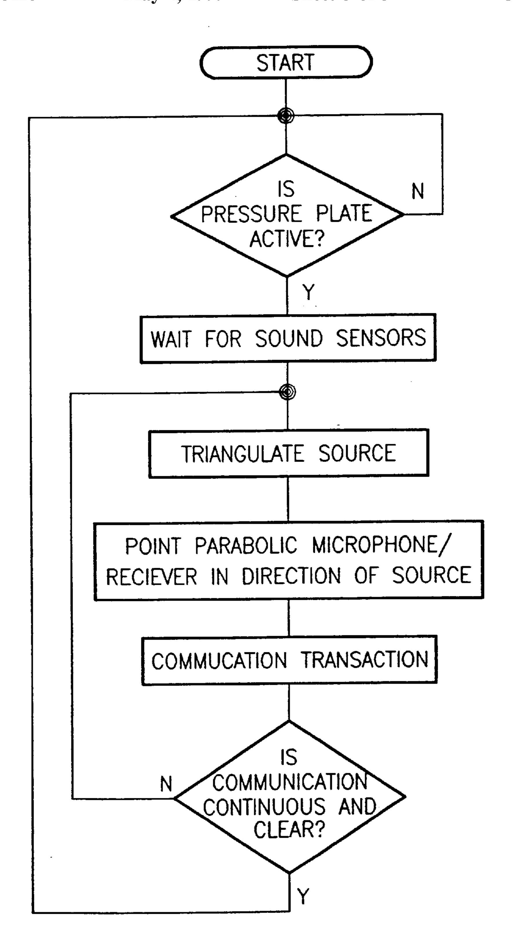
Fig. 4 Flow Chart for Processor
