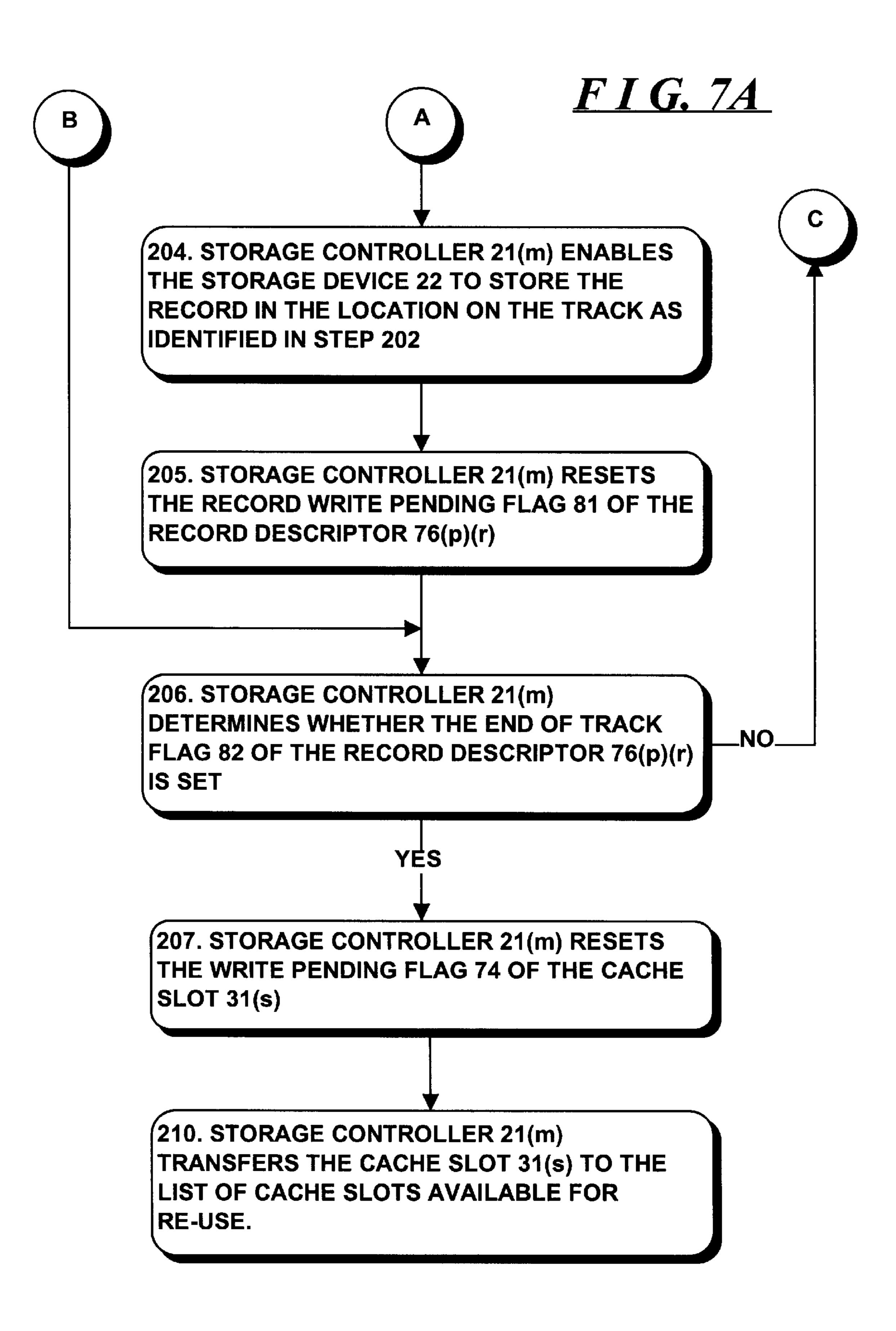
SYSTEM AND METHOD FOR ACCESSING RECORDS IN A CACHE SLOT WHICH ARE ASSOCIATED WITH A CURRENT OWNER STORAGE ELEMENT OR AT LEAST ONE PREVIOUS OWNER STORAGE ELEMENT
