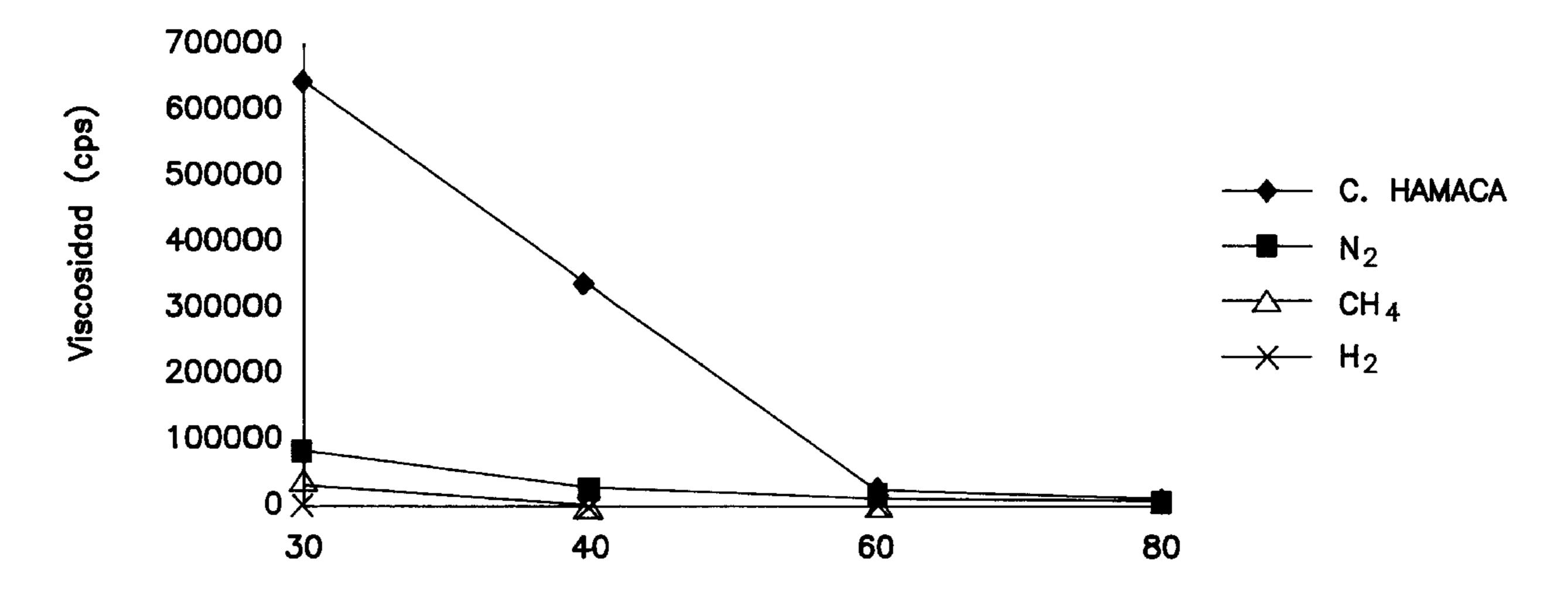
Temperature (°C) of the <u>viscosity measurement</u>
