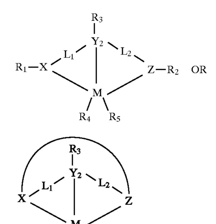
wherein M is a metal and R<sub>4</sub> and R<sub>5</sub> are each selected from the group consisting of halides and group 14 atomcontaining species such that X and Z each form an anionic bond to M and Y<sub>2</sub> forms a dative bond to M and the composition of matter has no net charge.
