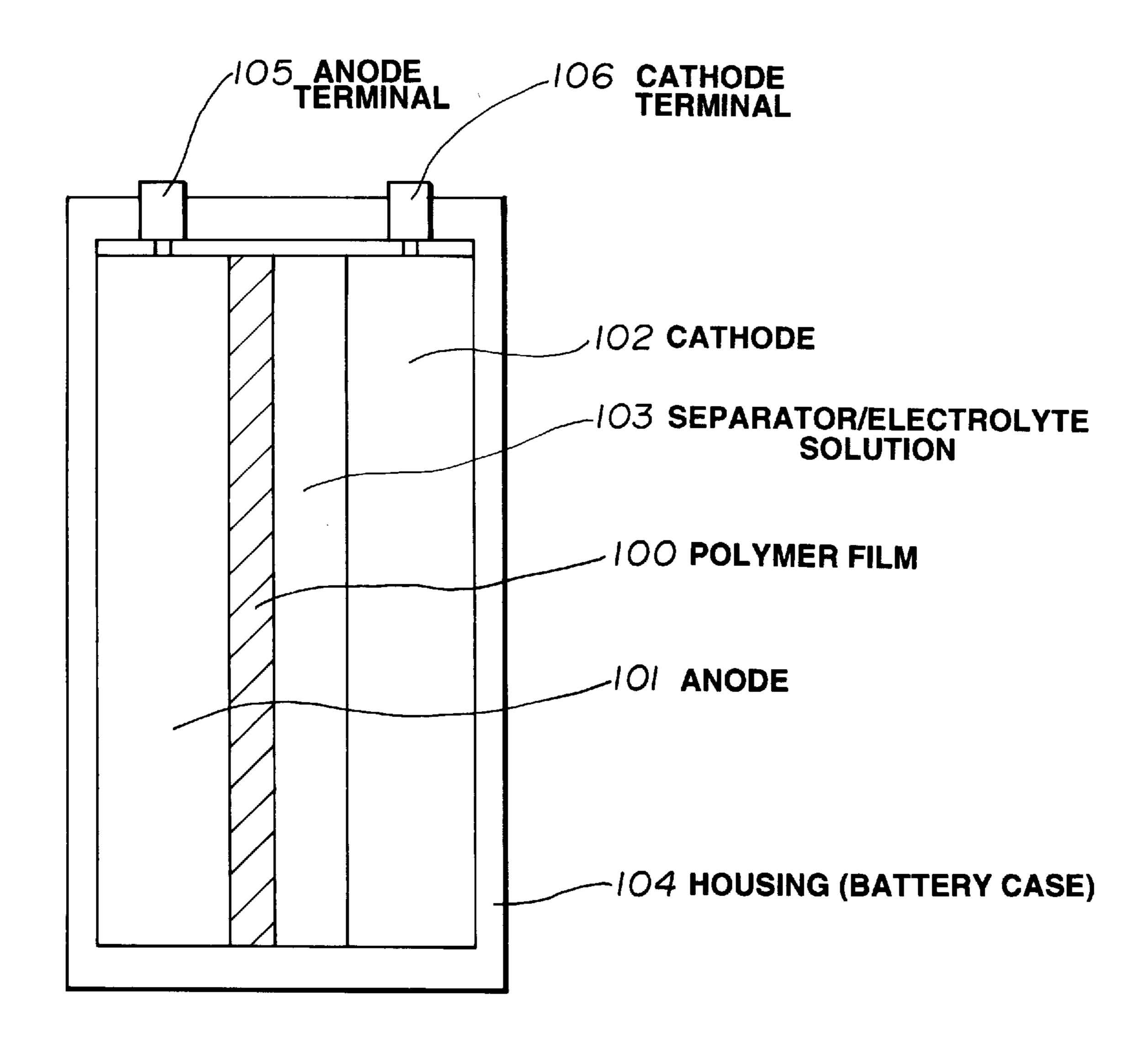
02 CATHODE ELECTROLYTE SOLUTION FIG.2(a) 100 POLYMER FILM O / ANODE 02 CATHODE 00 POLYMER FILM FIG.2(b) 03 SEPARATOR/ELECTROLYTE SOLUTION O/ ANODE 102 CATHODE 100a POLYMER FILM FIG.2(c) **ANODE**
