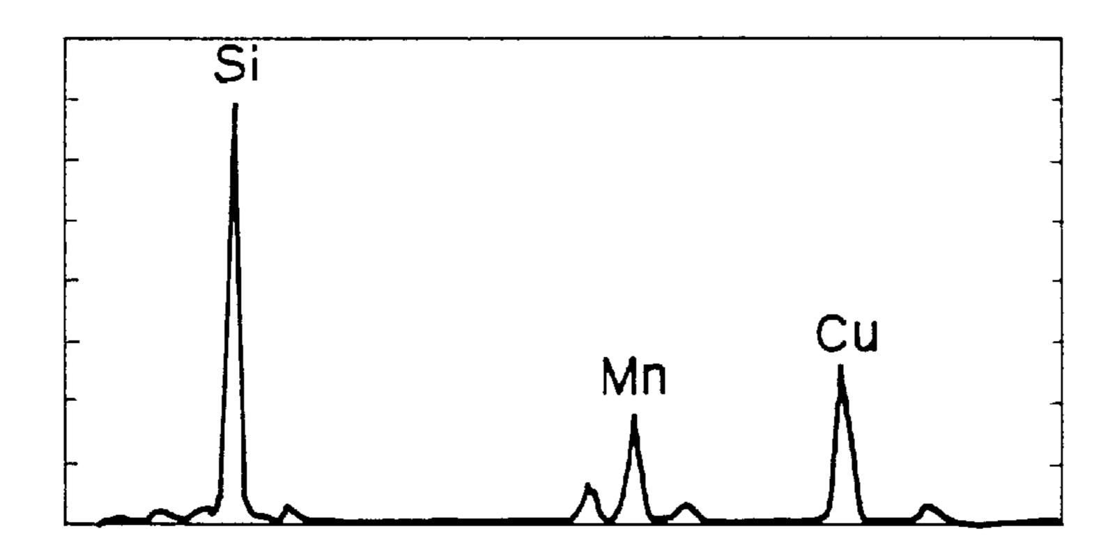
ELEMENT ANALYSIS: NEEDLE-SHAPED PRECIPITATED SUBSTANCE
