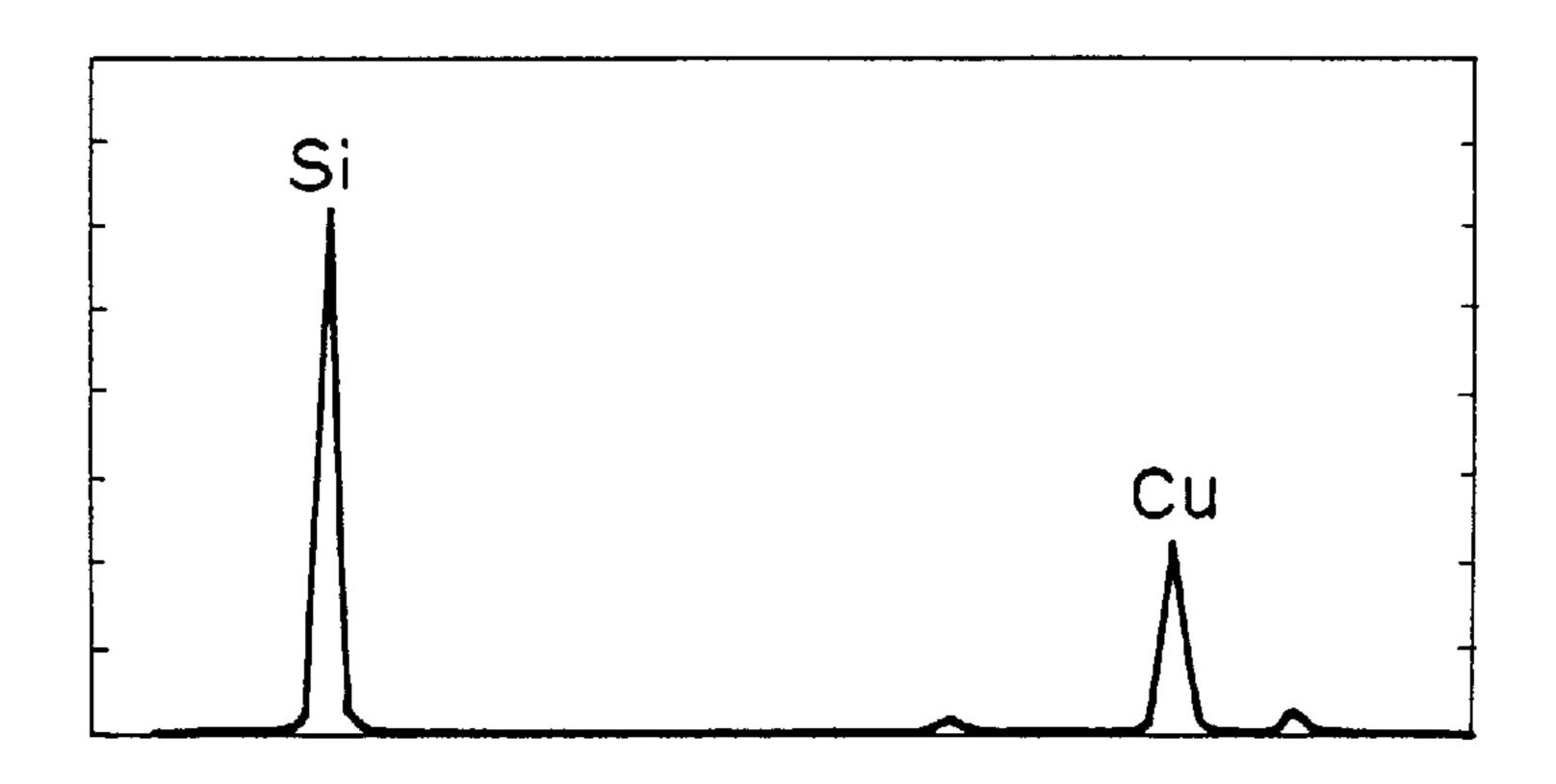
ELEMENT ANALYSIS: COARSE BLOCK-SHAPED PRECIPITATED SUBSTANCE
