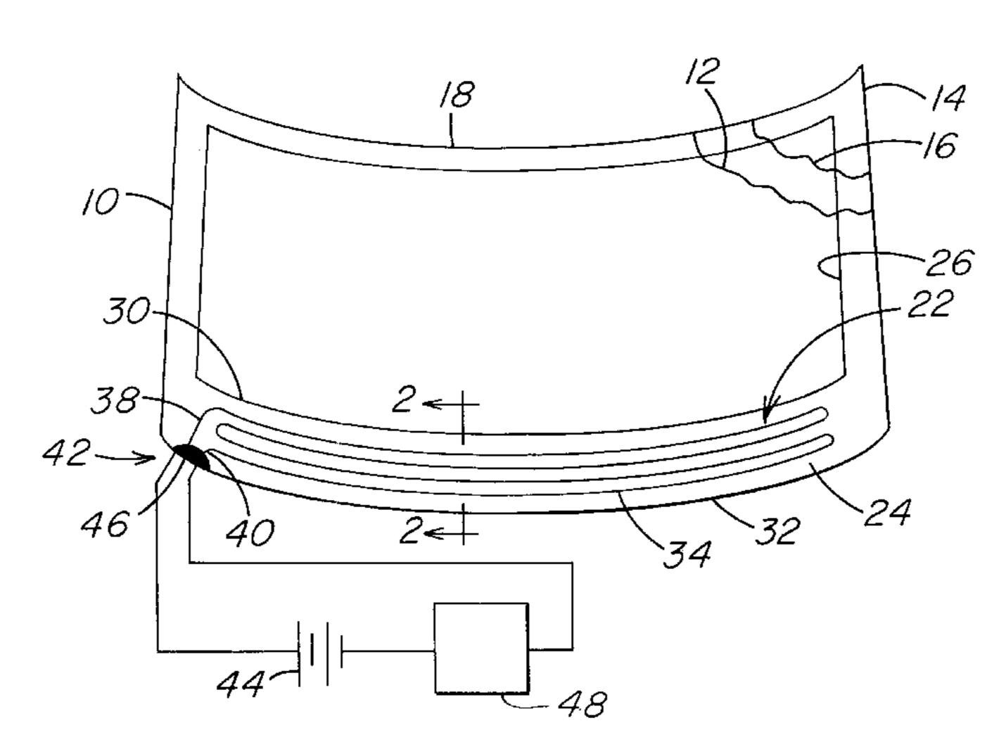
bonded to a major surface of the second glass sheet, which forms the inner ply of the windshield, along its marginal edge portion such that the wire is not visible when the windshield is viewed through the second glass sheet. In addition, the wire may include a coating having a color that generally corresponds to the color of the opaque ceramic band to mask the appearance of the wire when the windshield is viewed through the first glass sheet.
