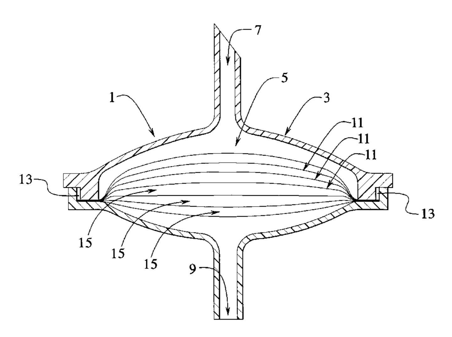
The invention provides a leukodepletion filter including a plurality of glass fiber filter pads, and a plurality of nonwoven polyester fiber filter pads, sealed within a filter housing.
