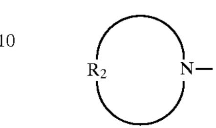
where each R<sub>1</sub> is independently selected from the group consisting of alkyls, cycloalkyls and aralkyls having from 1 to about 12 carbon atoms, and R<sub>2</sub> is selected from the group consisting of divalent alkylene, bicycloalkane, substituted alkylene, oxy- and N-alkylamino-alkylene group having from about 3 to about 16 methylene groups.
