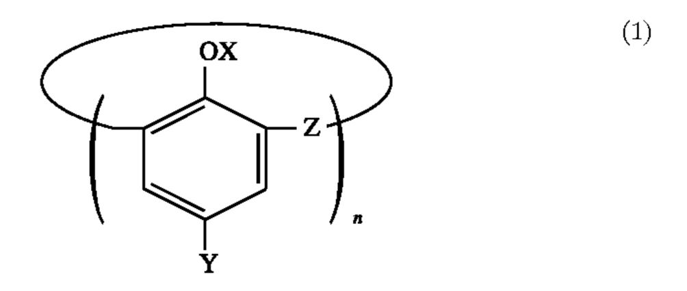
wherein X represents a hydrogen atom, a hydrocarbon group, an acyl group, a carboxyalkyl group, or a carbamoylalkyl group; Y represents a hydrocarbon group; Z represents a sulfide group, a sulfinyl group, or a sulfonyl group; and n is an integer of 4 to 8; and a method for extracting a transition metal using the composition
