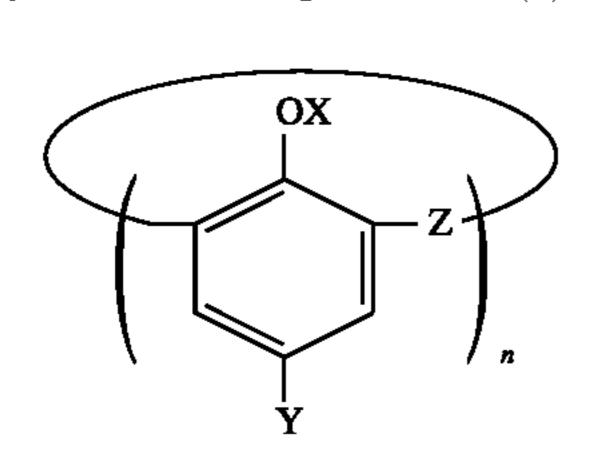
wherein X represents a hydrogen atom, a hydrocarbon group, an acyl group, a carboxyalkyl group, or a carbamoylalkyl group; Y represents a hydrocarbon group; Z represents a sulfide group, a sulfinyl group, or a sulfonyl group; and n is an integer of 4 to 8, and an extraction accelerator selected from the group consisting of basic nitrogencontaining heterocyclic compounds and aromatic amino acids.
