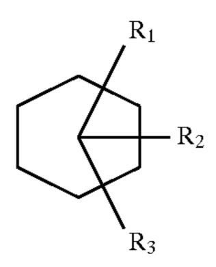
Group  $R_1$  is a linear or branched alkyl radical of formula  $C_nH_{2n+1}$  where n is greater than or equal to 1 and smaller than 25.
