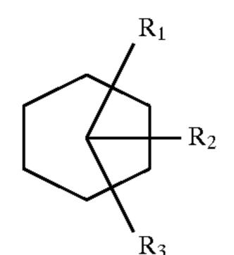
where group R<sub>1</sub> is a linear or branched alkyl radical of formula  $C_nH_{2n+1}$  where n is greater than or equal to 1 and smaller than 25, and where groups  $R_2$ ,  $R_3$  can be equal to or different from each other in a same molecule and can be H and/or linear or branched alkyl radicals of formula  $C_nH_{2n+1}$ where n is greater than or equal to 1 and smaller than 25.
