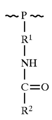
wherein P is a biocompatible polymer backbone having reactive functionality selected from the group consisting of isocyanates, carboxyls, amines, and mixtures thereof, and wherein said reactive functionality is independent of any urethane linkages present in said polymer back bone; R<sup>1</sup> is a hydrophilic spacer group selected from the group consisting of aliphatic hydrocarbons, poly(oxy olefins), hydrophilic polyethers, hydrophilic polyethylenes, modified polyolefins,
