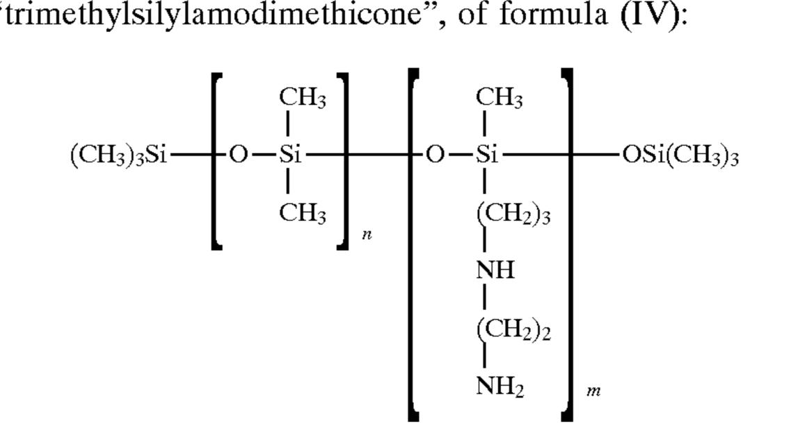
In this formula n and m are selected depending on the exact molecular weight of the compound desired.
