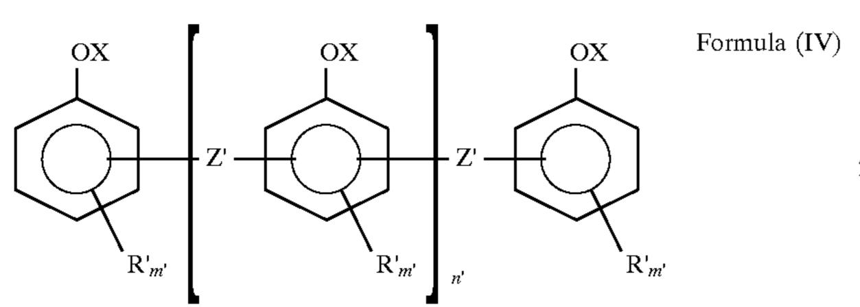
In the formula, R' each may be the same or different and is an alkyl group having 1 to 10 carbon atoms, a substituted or unsubstituted phenyl group, a substituted or unsubstituted aralkyl group, an alkoxy group or a halogen atom, Z' each may be the same or different and is a direct bond or a divalent hydrocarbon having 1 to 15 carbon atoms, n' is a number of from 0 to 2 on the average value, and m' each may 35 be the same or different and is an integer of from 0 to 4.
