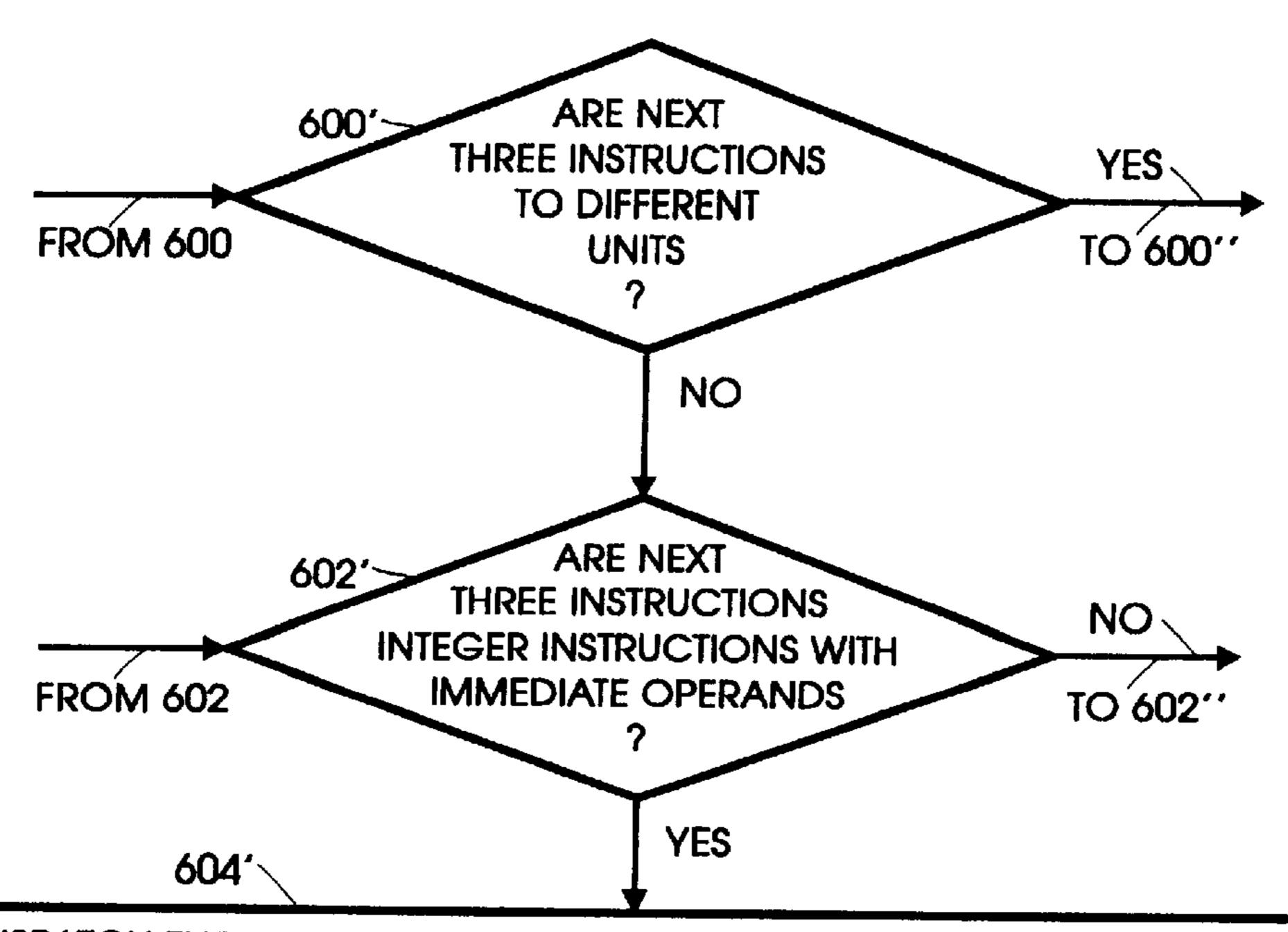
DISPATCH THREE INSTRUCTIONS IN SAME CYCLE: SEND FIRST INSTRUCTION TO FXU DECODER 112, SEND ITS IMMEDIATE DATA TO B-OPERAND REG 120, AND SEND FIRST GPR OPERAND TO A-OPERAND REG 122
