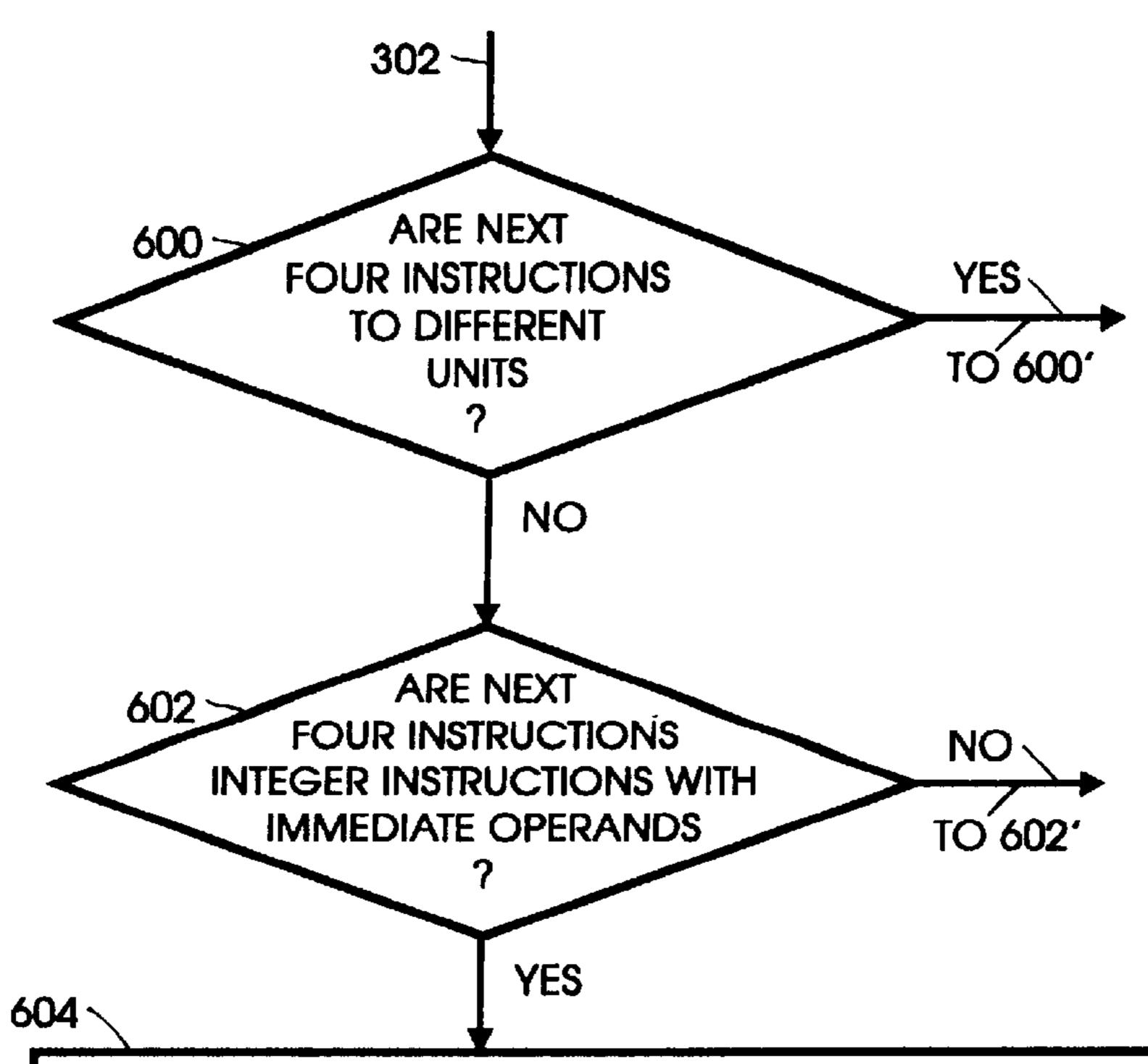
DISPATCH FOUR INSTRUCTIONS IN SAME CYCLE: SEND FIRST INSTRUCTION TO FXU DECODER 112, SEND ITS IMMEDIATE DATA TO B-OPERAND REG 120, AND SEND FIRST GPR OPERAND TO A-OPERAND REG 122
