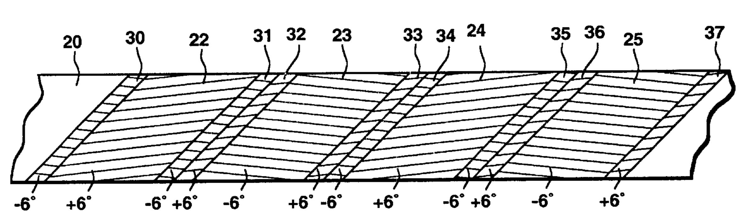
30 & 31 ARE A PAIR OF DUPLICATELY RECORDED TRACKS. 32 & 33 ARE A PAIR OF DUPLICATELY RECORDED TRACKS. 34 & 35 ARE A PAIR OF DUPLICATELY RECORDED TRACKS. 36 & 37 ARE A PAIR OF DUPLICATELY RECORDED TRACKS.
