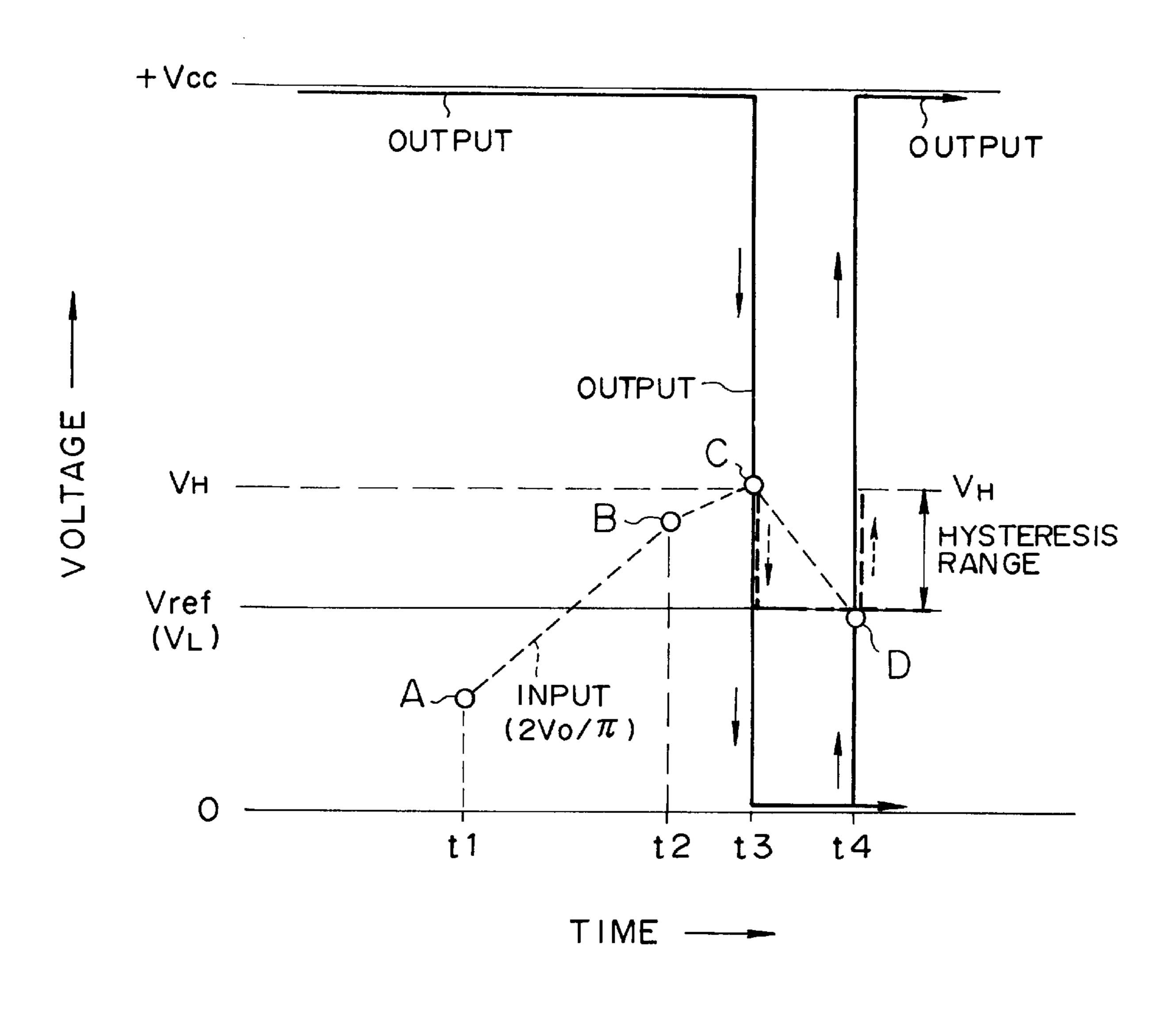
+INPUT TERMINAL FIG.9A VOLTAGE OF AMPLIFIER
