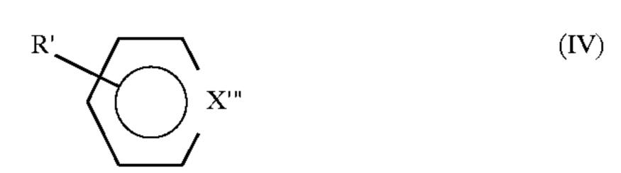
In the formula [IV], X" is nitrogen (N) or C—Y", wherein Y" is NH<sub>2</sub>, SO<sub>3</sub>H, CHO or COOH. That is, when X" is nitrogen, IV represents pyridine ring, when Y" is NH<sub>2</sub>, IV represents aniline ring, Y" is NO<sub>2</sub>, it represents nitrobenzene ring, Y" is SO<sub>3</sub>H, it represents benzenslufonic acid ring, Y" is CHO, it represents benzaldehyde ring, and Y" is COOH, it represents benzoic acid ring.
