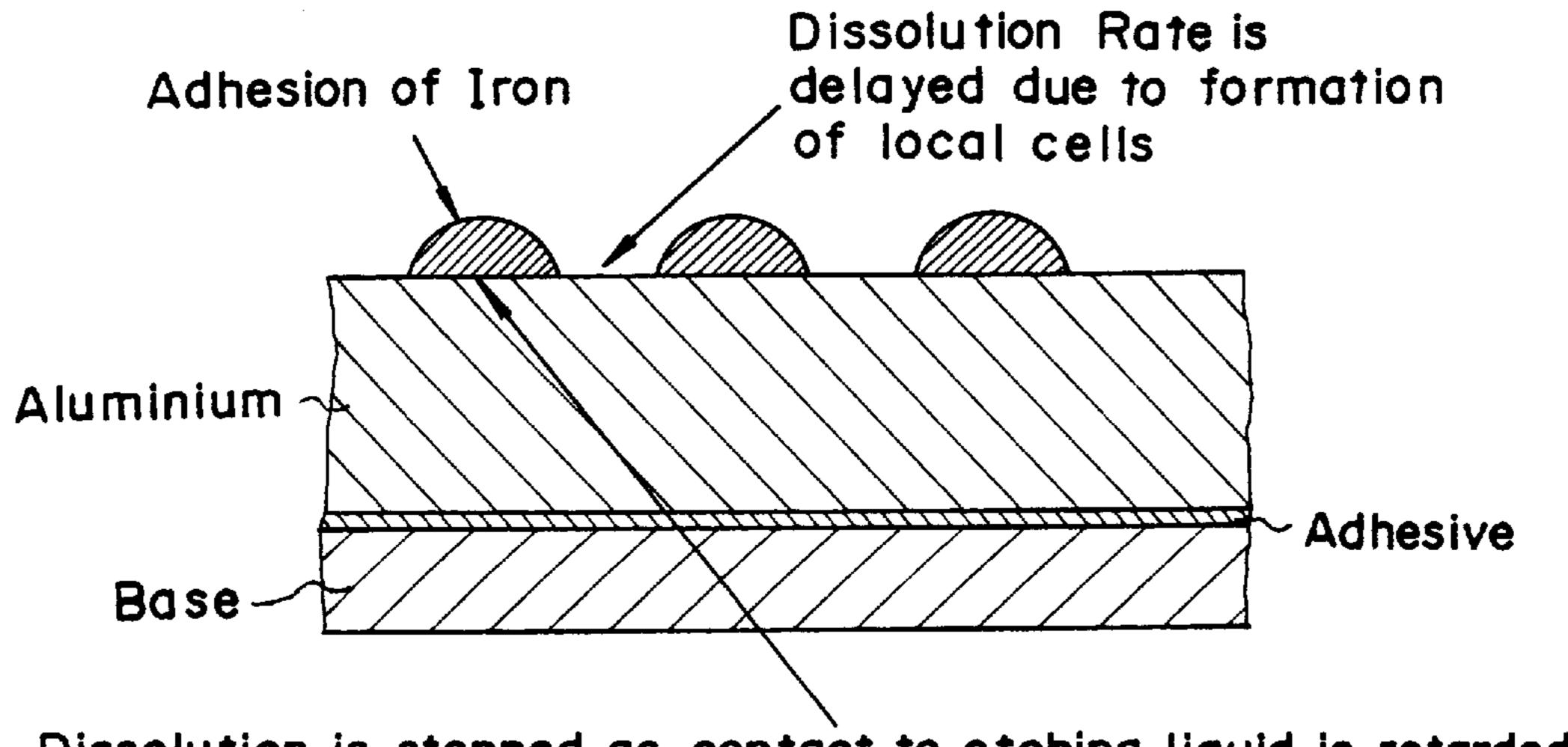
Dissolution is stopped as contact to etching liquid is retarded.
