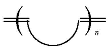
illustrates the structure of the resultant ring-opened polymerized unit with n being from 5 to 100,000.
